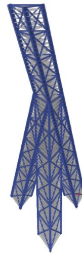
Figure 5.13: 3 mega columns with bracings, 270 m high
