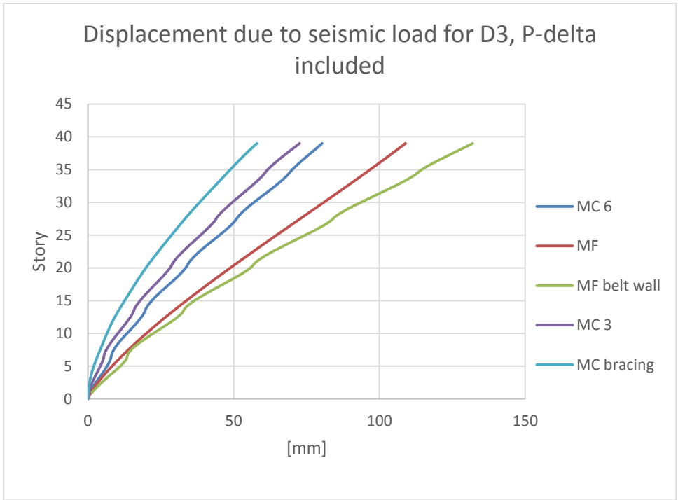
Figure B 21: Displacement due to seismic load in y-direction for diaphragm D3, P-delta included
