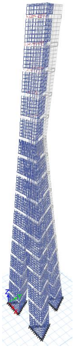
Figure A 33: Wind load deformation, X-direction
