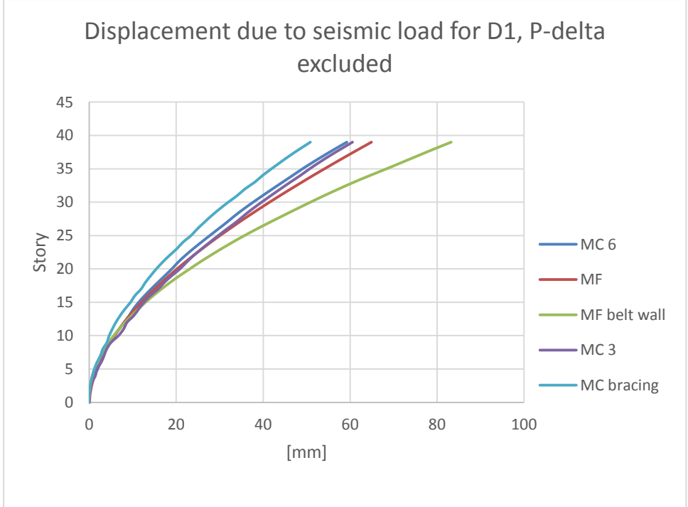
Figure B 22: Displacement due to seismic load in y-direction for diaphragm D1, P-delta excluded
