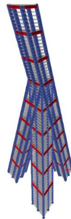
Figure 5.11: 6 mega columns with belt wall, 270 m high
