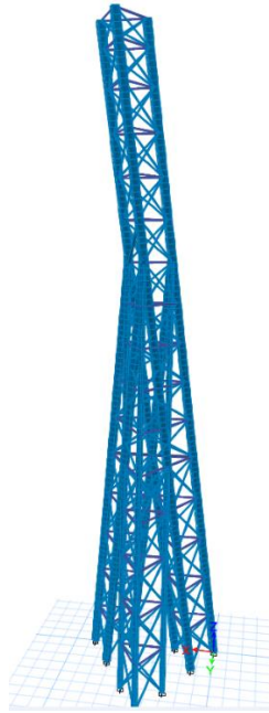
Figure 5.12: 3 mega columns with bracings, 450 m high
