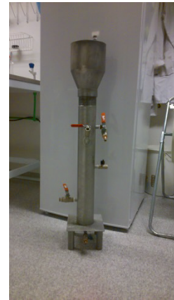
Figure 4. Ozone reactor customized for the wastewater treatability tests at Linnaeus University.
