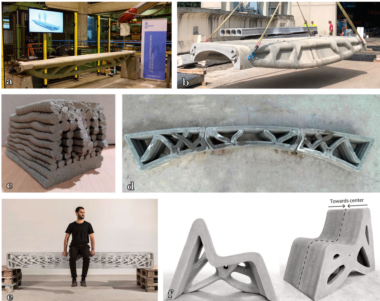
Figure 1. 3DCP projects incorporating structural optimisation: (a) Topology-optimised girder from Ghent University [16]. (b) Topology-optimised bridge from Ghent University [17]. (c) Functionally graded beam with TO from NTU Singapore [18]. (d) Topology-optimised 3DCP arch structure from Hebei University of Technology [19]. (e) Stress-based optimised beam from SDU [20]. (f) Topology optimised 3DCP structures from RMIT [13].
