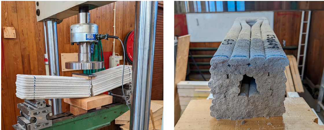
Figure 13. Testing of the 3DCP samples.
