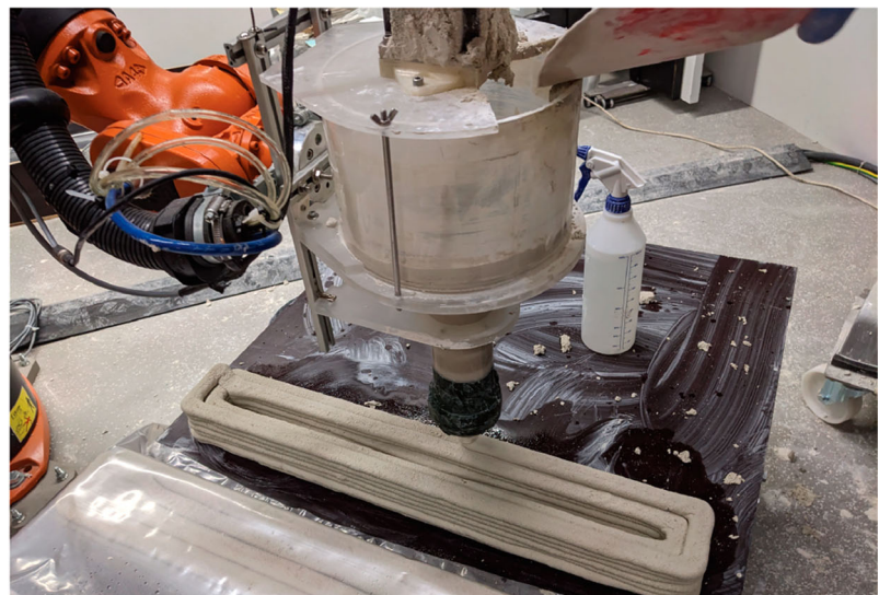
Figure 11. 3DCP robotic fabrication setup at the KTH School of Architecture.
