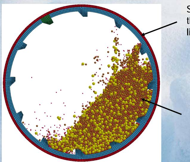
Structural parts of the mill (lifters, liners, shell) FEM
