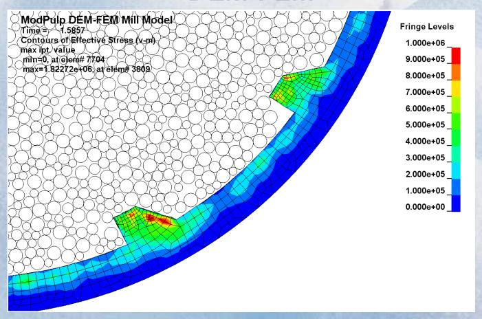
Charge level 25%, critical speed 73% (Von Mises Stress)
