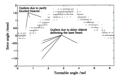
Figure 8: Raw measurement data, every dot represents the mean of the error angle at a certain turntable angle.
