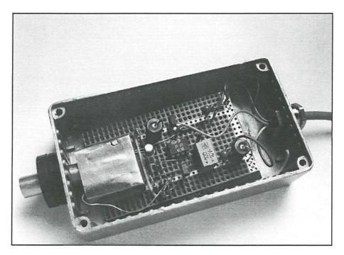
Figure 5: Photograph of the implemented PIF-circuit.
