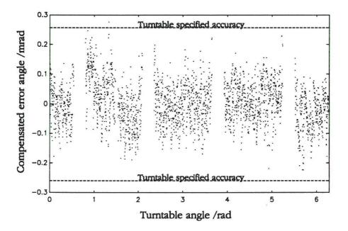
Figure 10: Error angle after removal of systematic errors.
