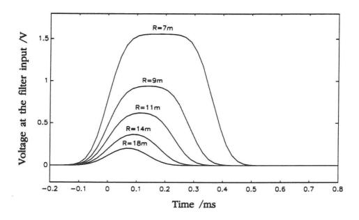
Figure 7: Numerically evaluated voltages at the filter input. The pulse shape goes gradually from the accumulated Gaussian distribution shape to the Gaussian shape when the laser beam expands with range.
