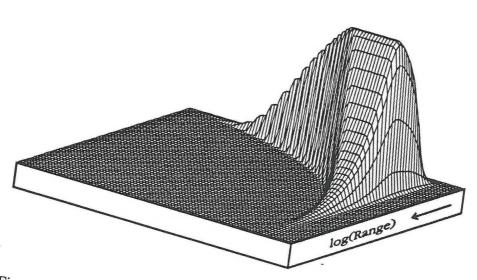
Figure 8: Two views of the voltage at the filter input as a funtion of time and range. The time interval is -0.5 ms to 4.8 ms and the range interval is 0.6 m to 60 m. The range axis is logarithmic.
