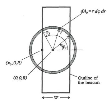
Figure 6: Area element on the beacon defining the integration limits  $\varphi_1$  and  $\varphi_2$ .
