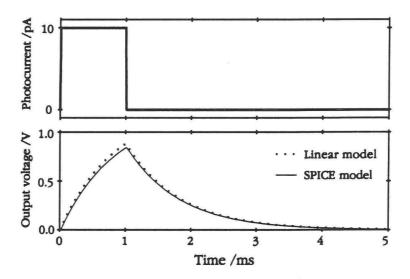
Figure 7: Pulse responses of the implemented PIF-circuit, given by the linear model and the SPICE model. Simulation results.
