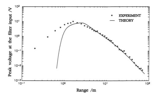
Figure 14: Experimental and theoretical peak voltage at the filter input. The descrepancy at short range is discussed in the text.
