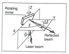
Fig 3 Coordinate system and symbols used to analyze the influence of the alignment error  $\beta$  on the measured angle error  $\Delta \gamma$
