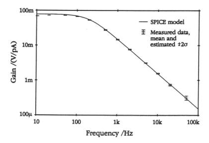
Figure 12: Magnitude of transfer function of the implemented PIF-circuit. The gain constant of the measured data has been adjusted to give a good fit with the simulated data, see the text. Measured and simulated data.
