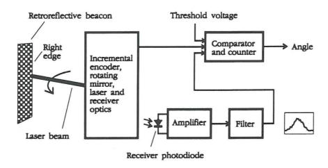
Figure 1: Block diagram of the anglemeter. Reflected radiation from the beacon hits a photodiode in the anglemeter receiver. An example of the received signal after the noise reduction filter is shown in the insert.
