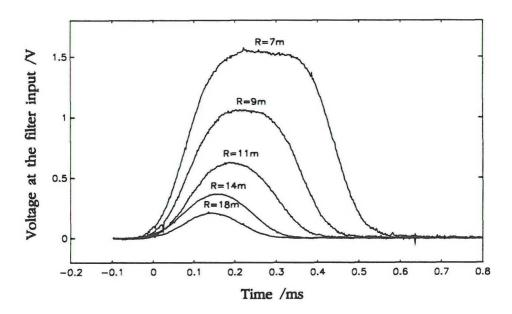
Figure 13: Measured voltage at the shaping filter input at R = 7, 9, 11, 14 and 18 m.
