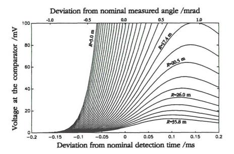
Figure 6: Numerically evaluated voltage at the comparator input for different range values. The angular deviation scale has been drawn using the constant angular velocity of the rotating mirror.
