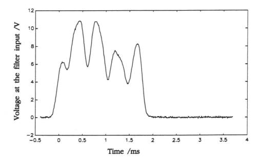
Figure 11: Measured voltage at the shaping filter input at R=1.4 m. The structure of the retroreflector is clearly resolved by the narrow laser beam.
