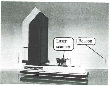
Figure 2: A photograph of the test vehicle Luleå Turbo Turtle (LTT). The length of the vehicle is about 1.2 m.
