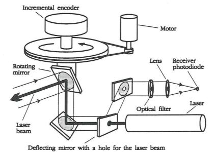
Figure 2: Optical part of the anglemeter. A small area in the center of the receiver aperture is wasted because it is occupied by the outgoing laser beam.
