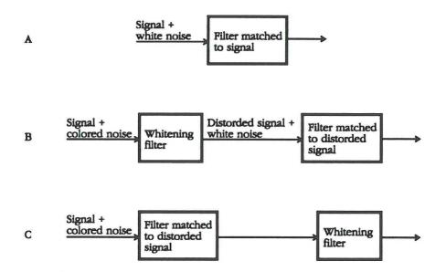
Figure 14: The signal-to-noise ratio is maximized whith a matched filter if the noise is white (A). A whitening filter is used whith colored noise (B). The sequence of the filters can be interchanged (C).
