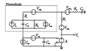
Figure 4: Noise equivalent circuit of the PIF-circuit. The symbols  $I_{nd}$ ,  $I_{na}$ ,  $V_{nR_s}$ ,  $V_{nR_1}$ ,  $V_{nR_2}$  and  $V_{na}$  denotes the noise generators in the PIF-circuit.
