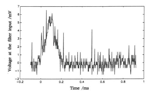
Figure 12: Measured voltage at the shaping filter input at R=70 m. The beam cross section is much larger than the beacon width at this range.
