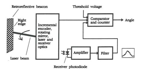
Figure 1: Block diagram of the anglemeter. Reflected radiation from the beacon hits a photodiode in the anglemeter receiver. An example of the received signal after the shaping filter is shown in the insert.
