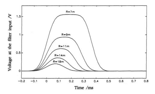
Figure 5: Numerically evaluated voltages at the input of the noise reduction filter. The pulse shape goes gradually from the accumulated Gaussian distribution shape to the Gaussian distribution shape when the laser beam expands with range.
