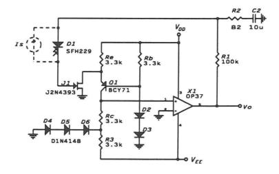
Figure 6: Circuit diagram of the implemented PIF-circuit. The current generator *Is* represents the photocurent in the photodiode.
