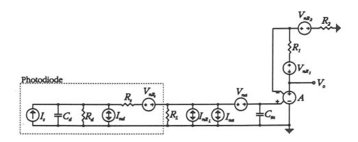
Figure 16: Noise equivalent circuit of the VA-circuit.
