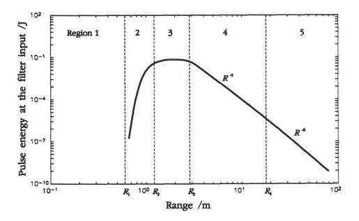
Figure 10: Numerically evaluated pulse energy at the shaping filter input. The different regions are described in the text.
