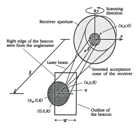
Figure 4: Definition of coordinate system and some symbols. All rays leaving the point (x,y,R) within the inverted receiver acceptance cone enters the receiver aperture with a sufficiently small incident angle to reach the photodiode.
