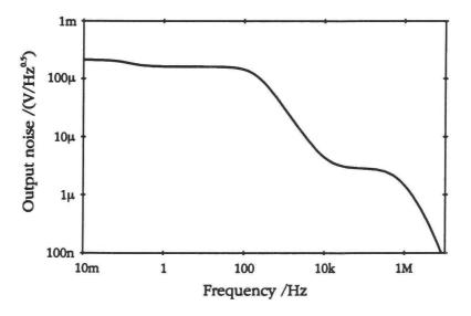
Figure 10: Output noise of the SPICE model of the implemented PIF-circuit. Simulation results.
