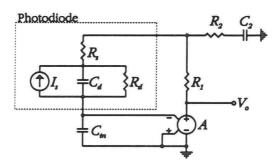
Figure 3: Small-signal equivalent model of the PIF-circuit. The photodiode is represented by the photocurrent generator  $I_s$ , the capacitor  $C_d$  and the resistors  $R_d$  and  $R_s$ . The input capacitance of the operational amplifier is represented by  $C_{in}$ .
