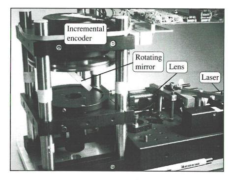
Figure 3: A photograph of the anglemeter. Note the pen in the bottom right corner for size reference.
