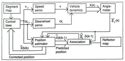
Fig 6. Block scheme over the different components in the navigation and control system.
