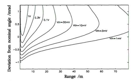
Figure 7: Deviation from nominal measured angle as a function of range with the threshold level of the comparator as parameter.
