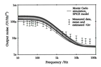
Figure 13: Output noise of the implemented PIF-circuit. Measured and simulated data.
