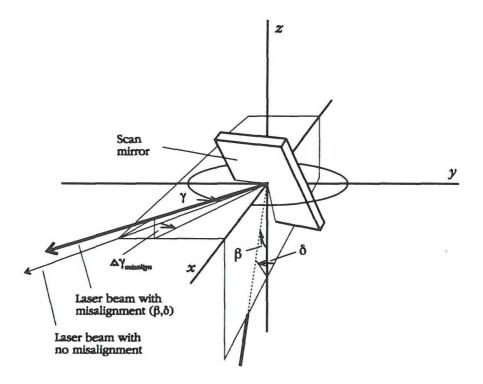
Figure 4: Coordinate system and symbols used to analyse the influence of the misalignment  $(\beta, \delta)$  on the measured angle  $\gamma$ .
