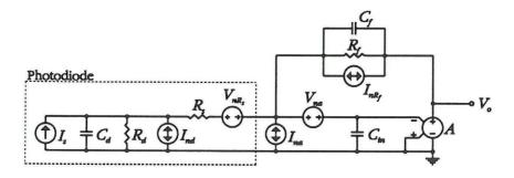
Figure 18: Noise equivalent circuit of the TIA-circuit.
