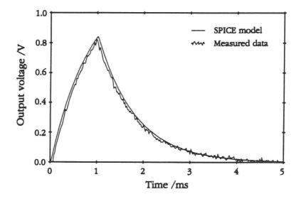
Figure 11: Pulse response of the implemented PIF-circuit. Measured and simulated data.
