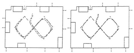
Fig 9.The estimated and simulated trajectory differs when no angles are used for the update of the position.
