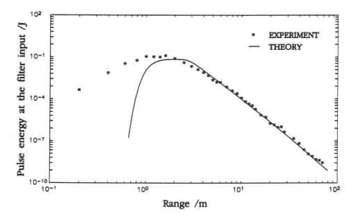
Figure 15: Experimental and theoretical pulse energy at the filter input. The descrepancy at short range is discussed in the text.
