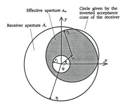
Figure 5: The receiver aperture. The shaded area marks the effective aperture for a point on the beacon. The point is at distance r from the optical axis.
