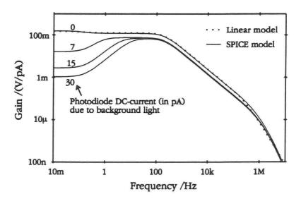
Figure 8: Magnitudes of the transfer function of the SPICE model of the implemented PIF-circuit. The pole with the lowest frequency and the gain constant of the transfer function are dependent on the bias point of the photodiode. Simulation results.
