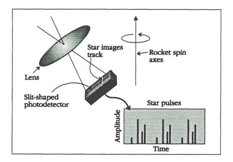
Figure 1: Principal drawing of star sensor optics. The shown pulse-pattern is generated by four stars during three spin-periods.
