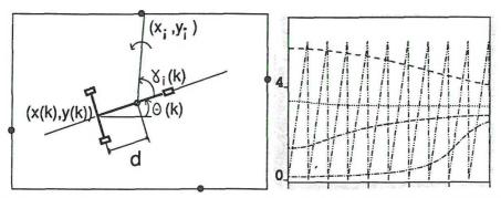
Fig 5. Principle of angular measurements and variation in the angles to four reflectors when the vehicle follows a straight line with the speed  $0.5 \, \text{m/s}$ .
