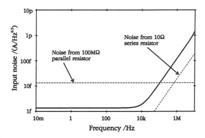
Figure 9: Input noise of the SPICE model of the implemented PIF-circuit. Noise contributions from a small resistor in series with the photodiode and from a large resistor in parallel with the photodiode are also shown for comparison. Simulation results.
