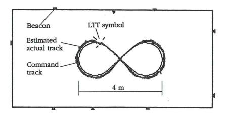
Figure 4: First successful run with the LTT. The rectangle represent our lab (6x12 m<sup>2</sup>) and the triangles indicate beacons. The inner path is the set-path and the outer zaggy curve is the vehicles recording of its track.
