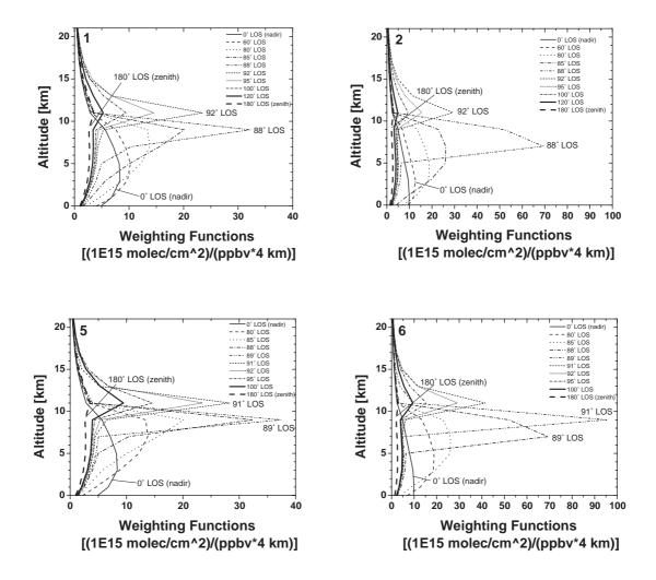
Fig. 3. Weighting functions for the scenarios 1, 2, 5, and 6. The NO<sub>2</sub> profile is anticipated for mid-latitudes on the northern hemisphere in March at 51.6° SZA. Each weighting function corresponds to a different LOS. The magnitude of the weighting functions is small at the surface and above 15 km, revealing that the slant columns are not very sensitive to NO<sub>2</sub> in these regions.
