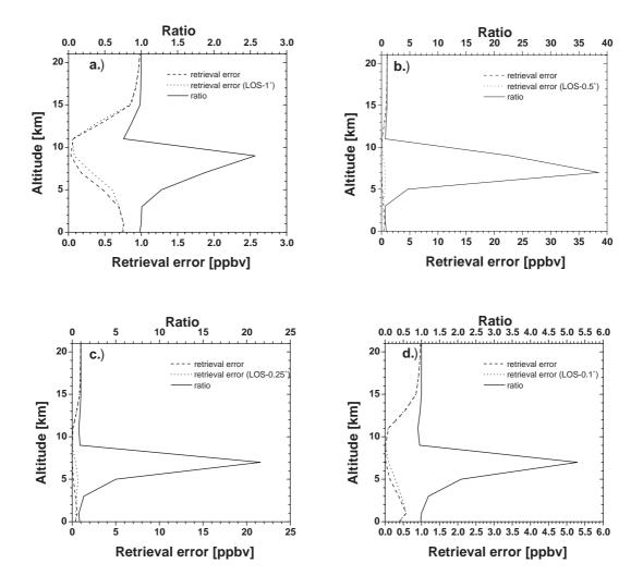
Fig. 7. Pointing accuracy: a.) pointing error of -1° for scenario 9, b.) pointing error of -0.5° for scenario 10, c.) pointing error of -0.25° for scenario 10, and d.) pointing error of -0.1° for scenario 10. To characterize the decrease in quality of the retrieval the ratio of the retrieval error with and without pointing error is plotted.
