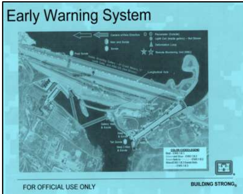
Fig 7: Early warning system showing locations of instruments and cameras
