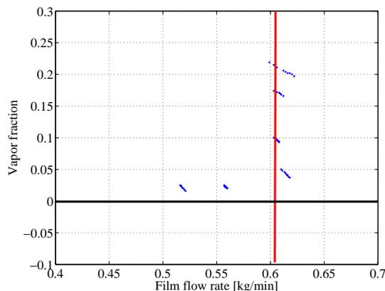
FIGURE 2.5. Example of suction curve from the experiments. The film flow rate is determined from the intersection of the vertical part of the curve with the horizontal axis.
