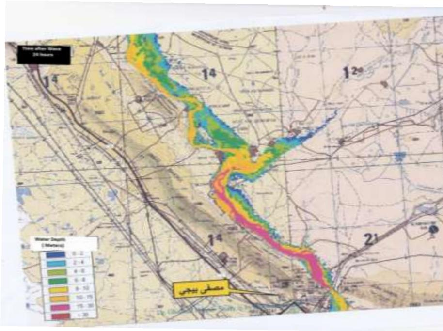
Figure 10: Wave at Makhul (Just North of Baije) after 36 hours of Dam Break
