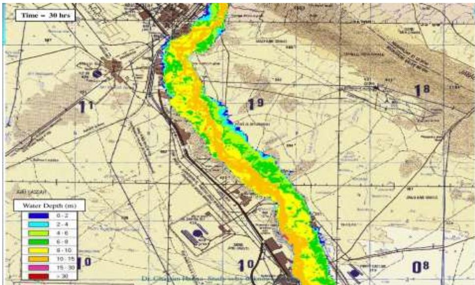
Figure 11: Wave at Tikrit after 24 hours of Dam Break
