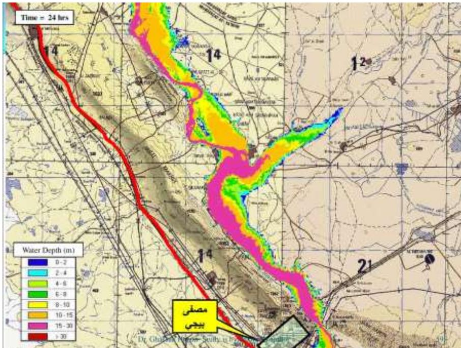
Figure 9: Wave at Makhul (Just North of Baije) after 24 hours of Dam Break
