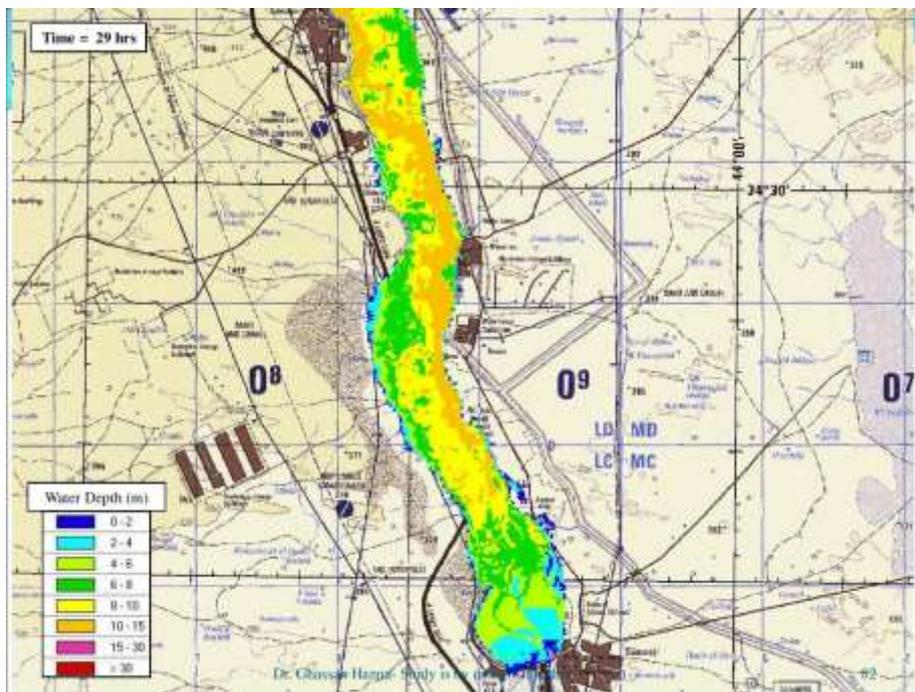
Figure 13: Wave at Sammara after 29 hours of Dam Break
