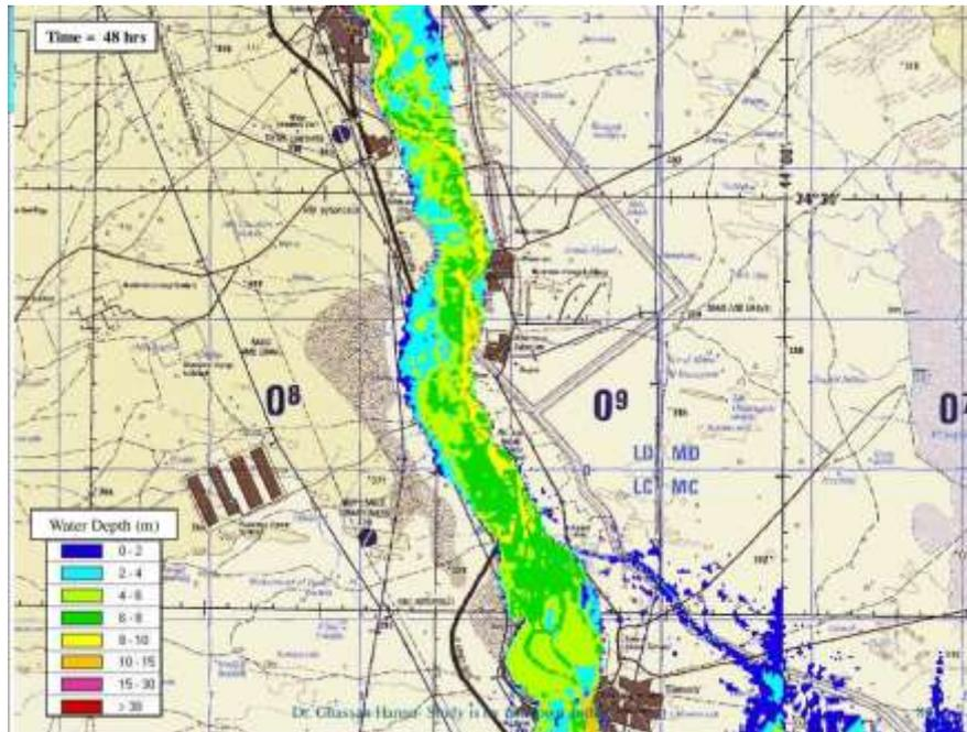
Figure 14: Wave at Sammara after 48 hours of Dam Break.
