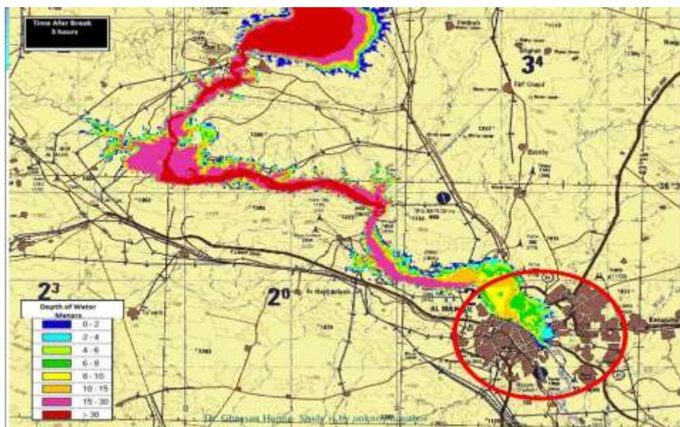
Figure 7: Flood wave at Mosul after 3hours of Dam break and various depths of inundation are explained by the colored legend.
