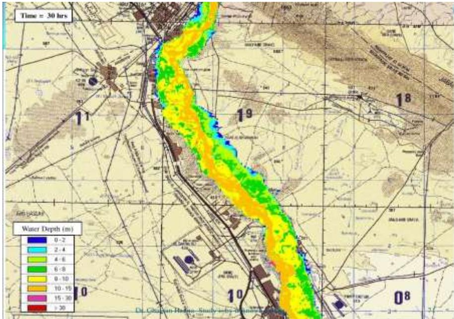
Figure 12: Wave at Tikrit after 30 hours of Dam Break
