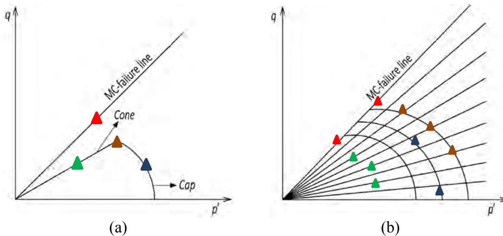
**Figure 14:** Plastic points at Hardening soil model
