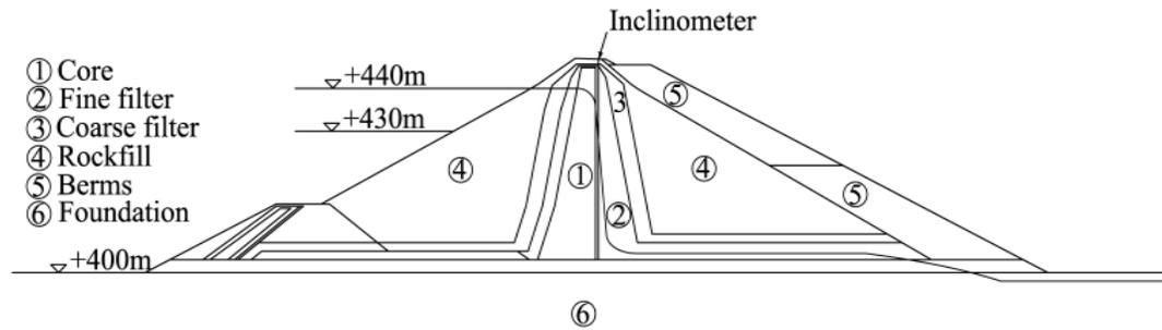
**Figure 1:** Cross section of the dam
