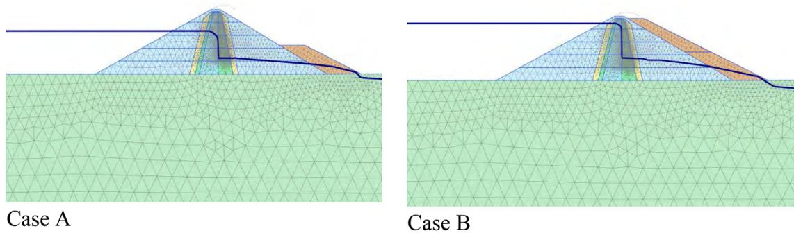
**Figure 2:** Finite element model of the dam for case A and case B
