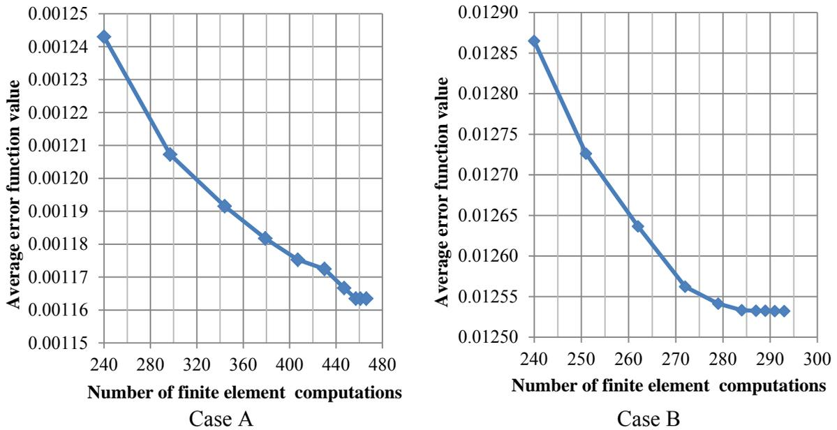
**Figure 12:** Average error function values versus number of finite element computations for the reduced search domain
