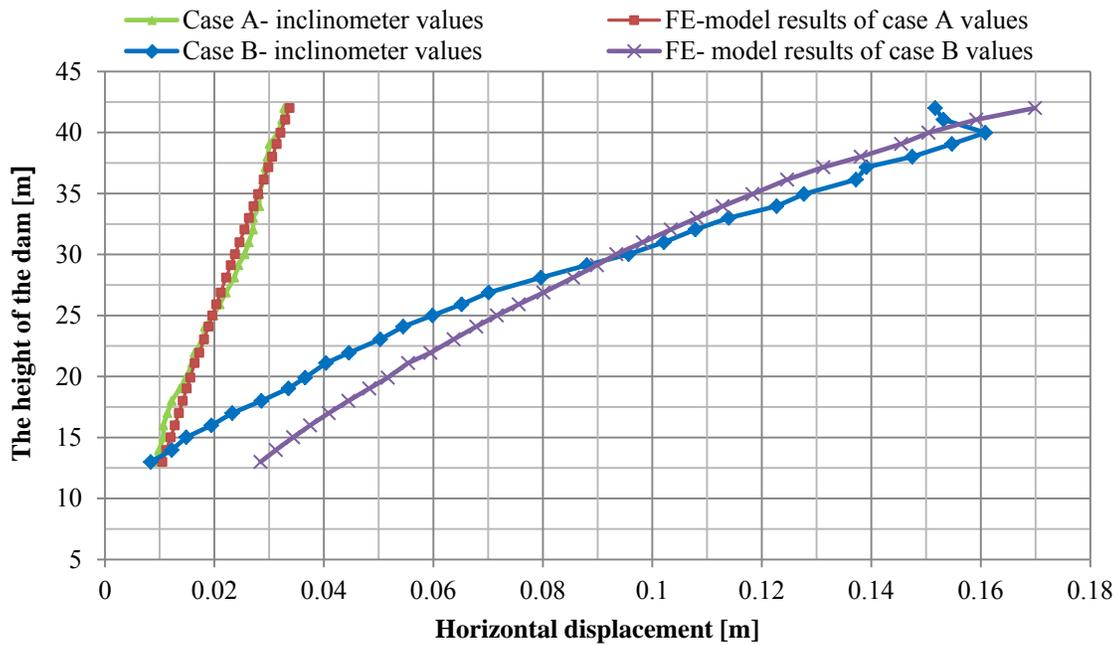
**Figure 11:** Measured and computed horizontal displacements at different heights of the dam for cases A and B
