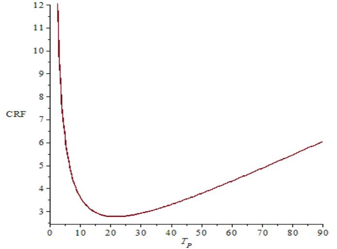
Figure 2: Cost rate vs. optimal inspection interval
