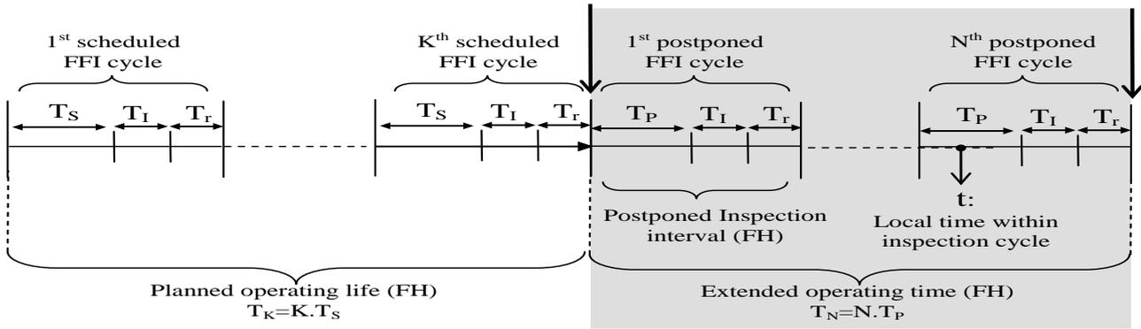
Figure 1: Schematic description of inspection and discard cycles
