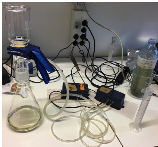
Figure 18. Filtration of a water sample. The sample can be seen in the plastic bottle to the right. The blue boxes in the middle of the picture are the vacuum pumps and the filtration unit is to the left. The filtered sample was collected in the big glass jar and was later transferred to plastic bottles.
