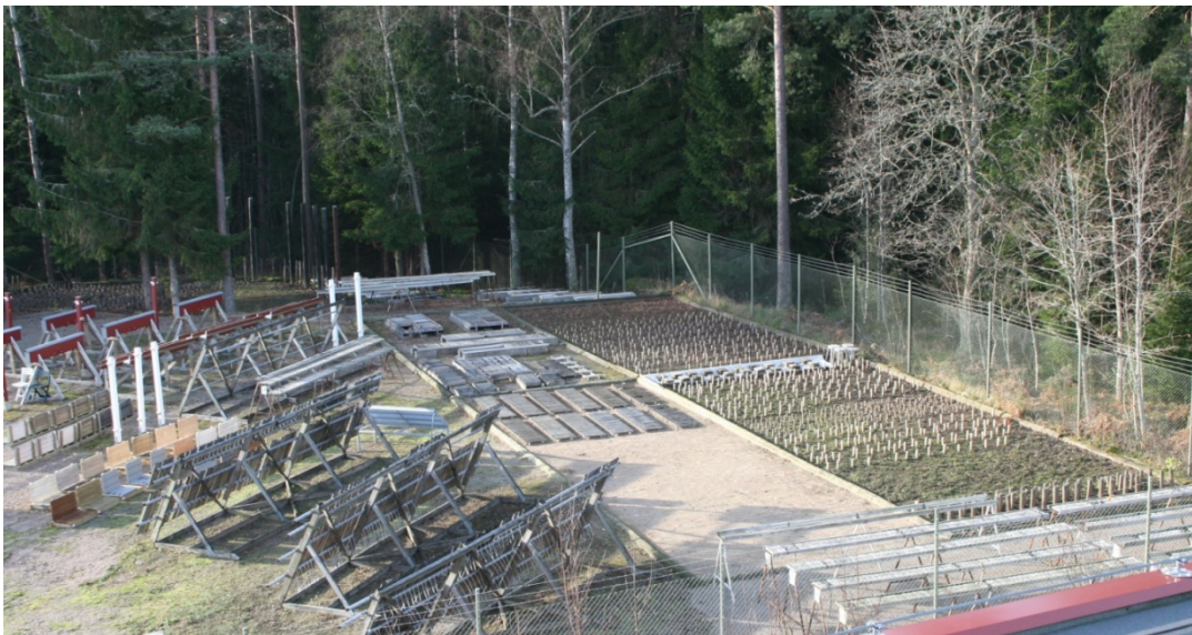
Figure 14. How can early results from field trials be used to predict the performance of a wood product? SP test site in Borås, Sweden.
