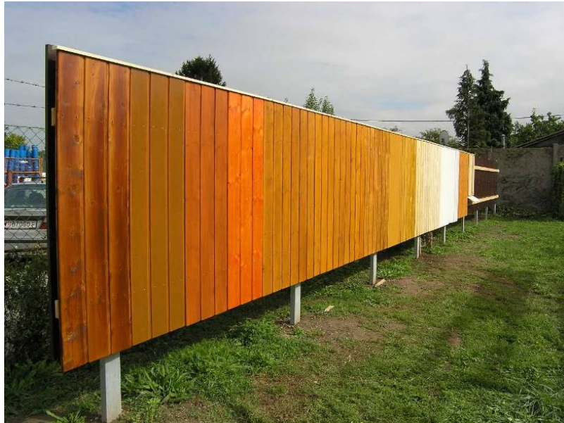
Figure 21. Natural weathering exposure of south west oriented vertical cladding in Vienna.
