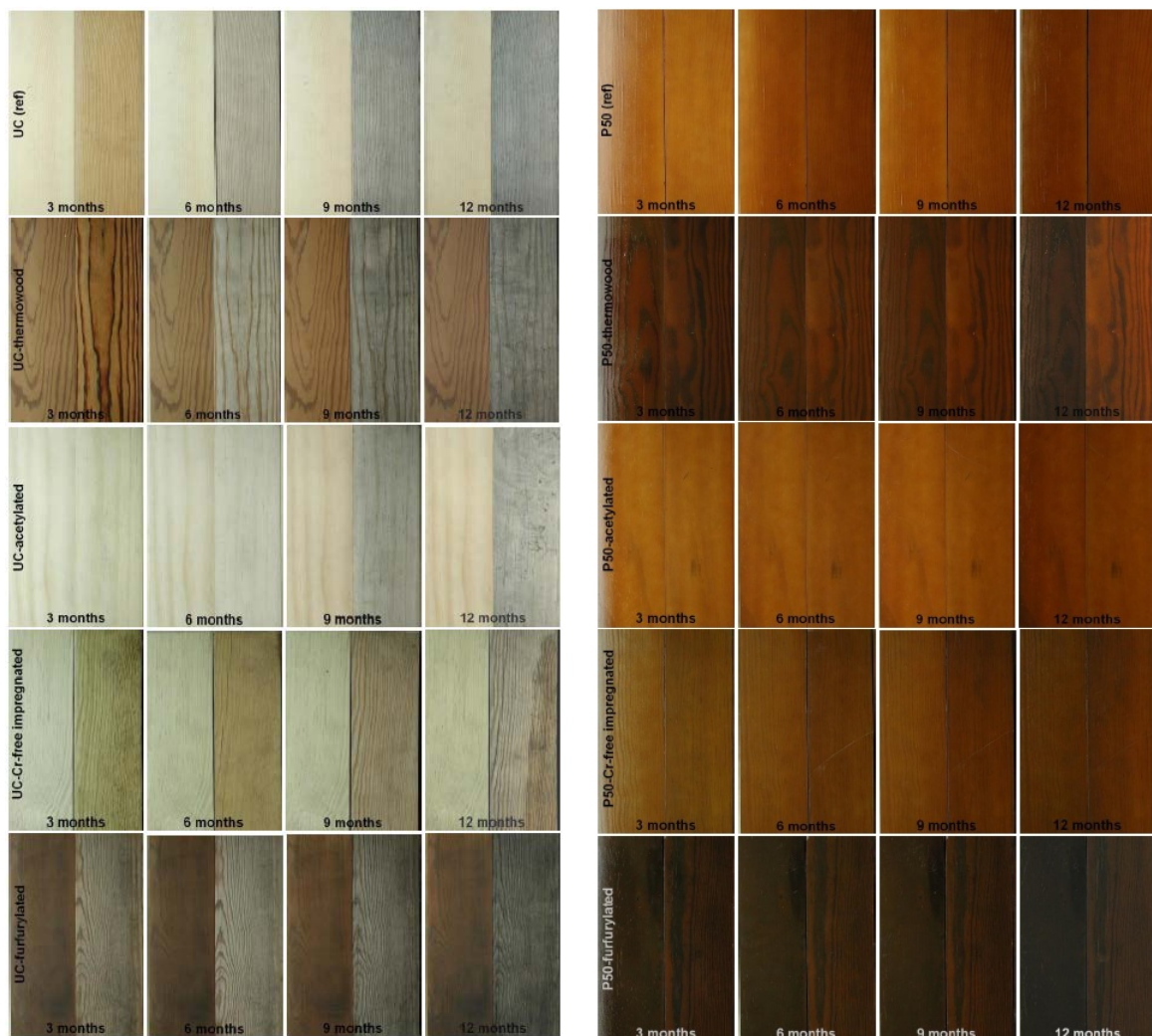
Figure 20. Pictures of uncoated and coated samples with different wood modification methods; unexposed reference (left) and panel after natural weathering exposure (right).
