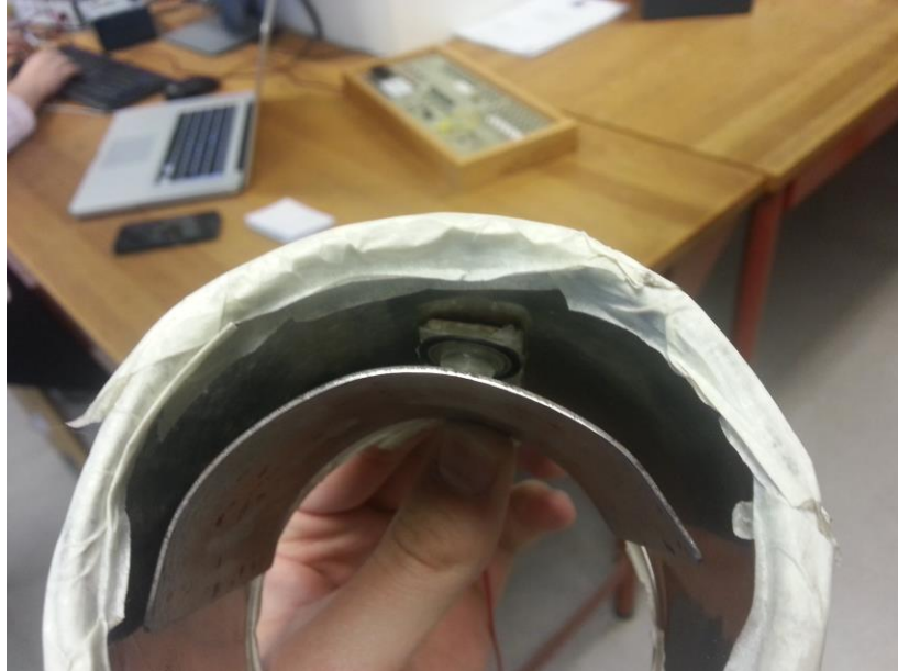
Figure 3.5. The metal ring prototype with pressure pads. Between the two metal parts is the force sensor placed.
