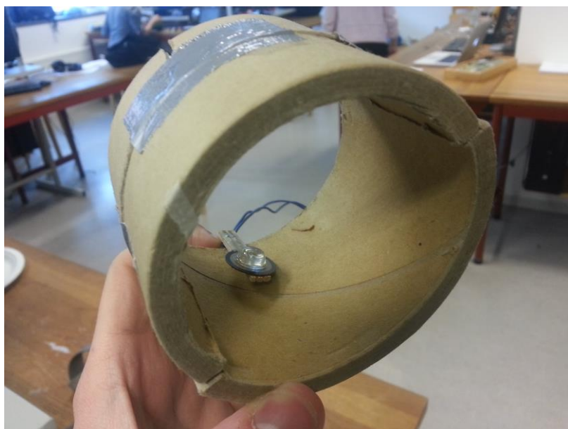
Figure 3.4. The paper ring prototype with the force sensor at the bottom of the inside. The other sensor is placed on the upper half of the ring.
