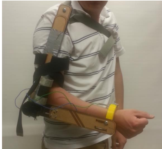
Figure 3.8. An image showing the demonstrator. The black part on the joint between the upper and lower arm is the motor and worm gear. The yellow part is the sensor mount.
