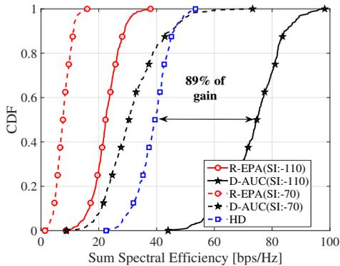
Figure 3. CDF of the sum spectral efficiency among all users for different SI cancelling levels. We notice that with  $\beta = -110$  dB the UE-to-UE interference is the limiting factor, where D-AUC mitigates this new interference and outperforms the HD mode and the R-EPA. When  $\beta = -70$  dB, the SI is the limiting factor, where the mitigation of the UE-to-UE interference is not enough to bring gains to FD cellular networks.
