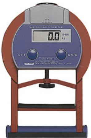
**Figure 1** T.K.K. 5401 GRIP D handheld dynamometer. (<http://www.takei-si.co.jp/en/productinfo/detail/49.html> Retrieved 2016-03-22)
