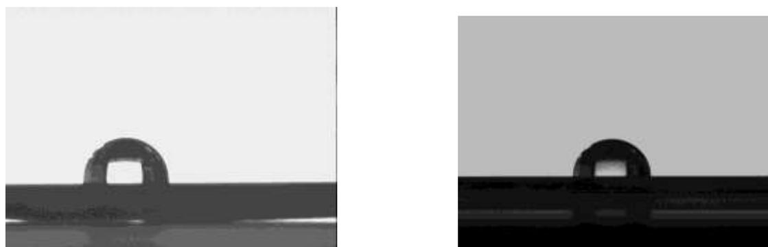
**Figure S6.** Water contact angle pictures for PS thin film giving a value of 95° (left) and for DB-TTF/PS blend thin film with a value of 91° (right). The pictures point towards hydrophobic surfaces for both cases.
