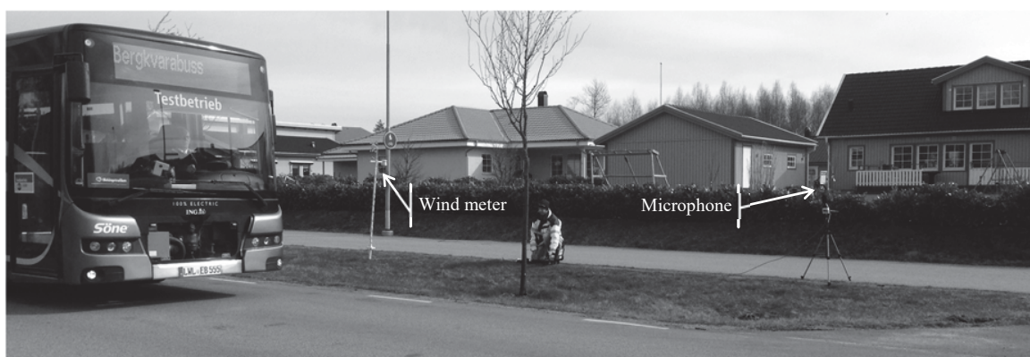
Fig. 2 Noise measurement of the electric bus when driving 30 km/h. Photo: Sven Borén
