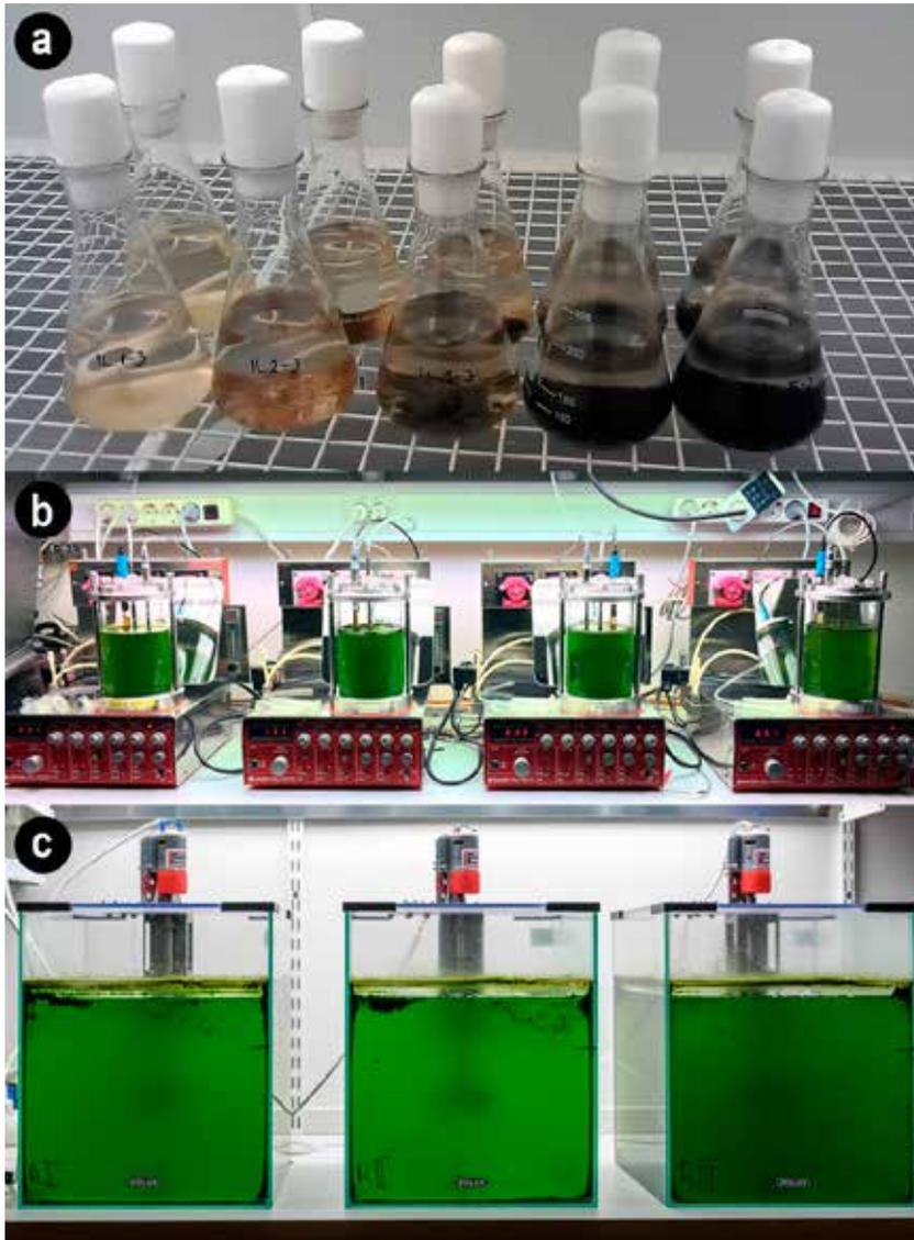
**Figure 5.** 250 ml flasks used in the proof of concept (Paper I) experiments (a), 1L photobioreactors used in the experiments studying the effect of lake water inoculation (Paper I) and nitrification inhibition (Paper II) on algal growth (b) and 20L photobioreactors designed and built to study the bacterial and algal community and functional genes (Papers III and IV) in lake water inoculated and uninoculated reactors (c).
