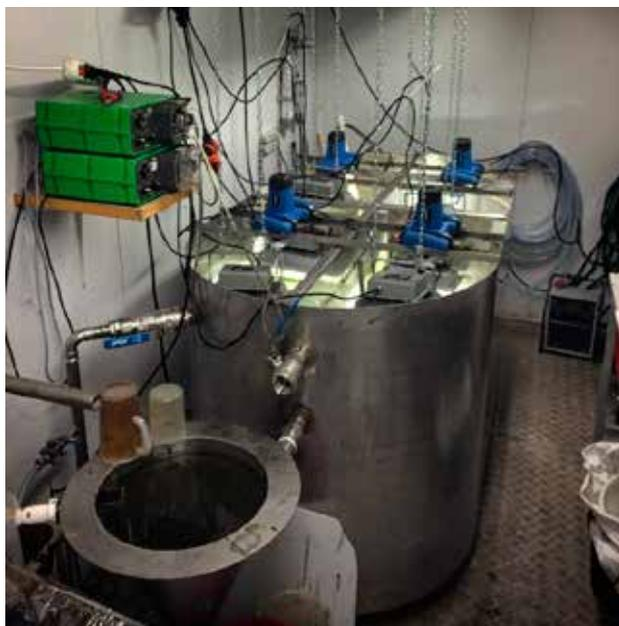
**Figure 1.** Experimental wastewater treating photobioreactor system combining microalgae with the activated sludge process in Västerås wastewater treatment plant, Sweden.
