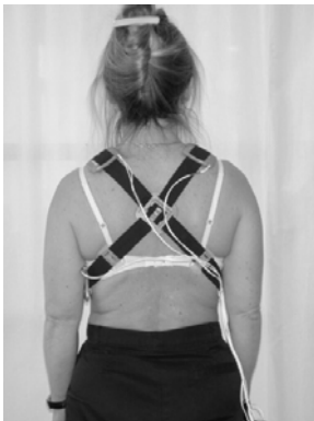
Figure 6. Individual in the myofeedback training group wearing a harness with electrodes over the trapezius muscle in the straps. The EMG logger and feedback device is carried in a small pouch/bag.
