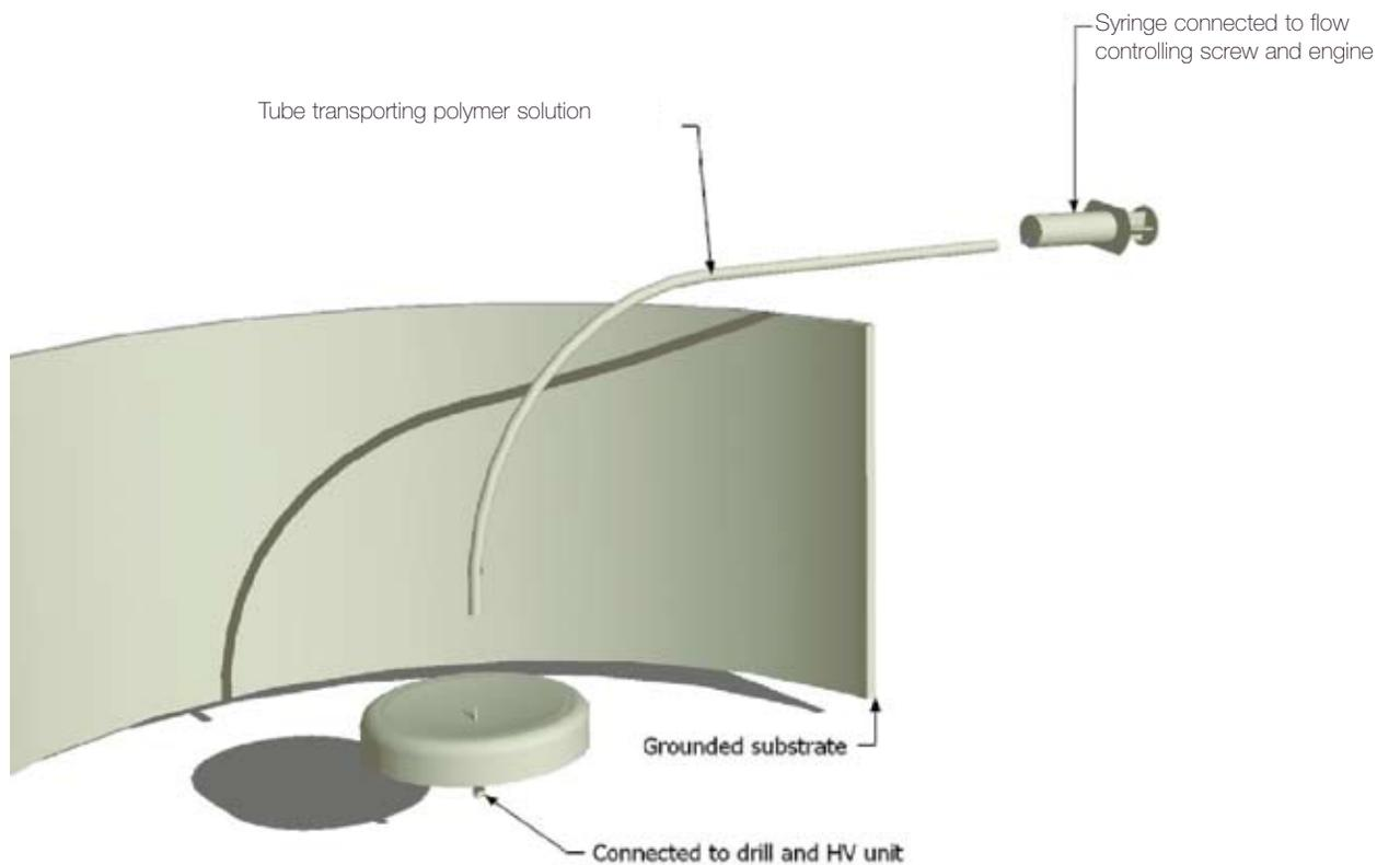
Figure 1. Principle sketch of the large-scale electrospinning device developed at IFP RESEARCH AB [2].
