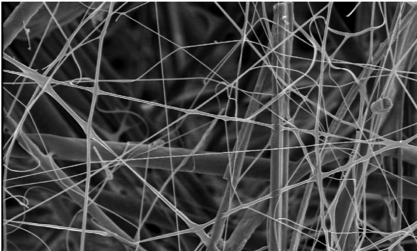
Figure 6. PVA electrospun on a non-woven substrate of cellulose. The fibers of the substrate have diameters in the range of 2-10  $\mu\text{m}$ , while the PVA fibers have diameters in the range of 200-700 nm.
