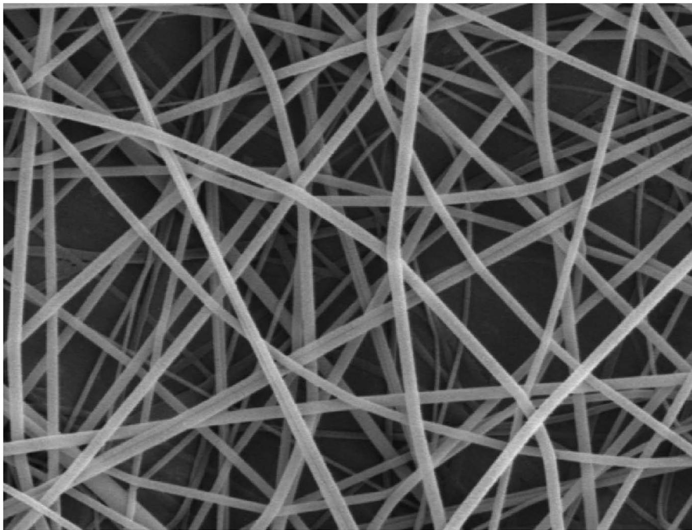
By cross-linking the polymer chains within the fibers dissolution of the web could be prevented. However, although the cross-linked PVA-web withstands water, swelling temporarily turns the fibers into a film. By soaking the film in organic solvents the fiber structure can be restored. This procedure is shown in Figure 4 a, b and c. Work is in progress to increase the degree of cross-linking in order to prevent film formation.
