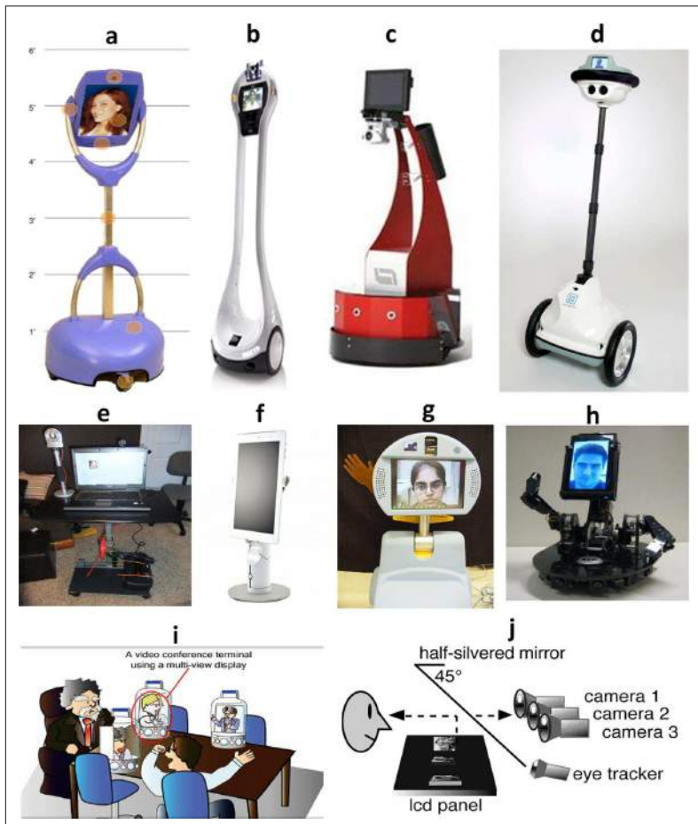
Fig. 2.2: Non-anthropomorphic video conferencing systems: [(a) Giraff (b) VGO (c) TiLR (d) QB are mobile robotic telepresence system (MRP) system with LCD, webcam, monitor and added capability of mobility [86].] (e) Embodied Social Proxy [ESP] by Microsoft for video teleconferencing [137]. (f) 2DOF of neck robot for video conferencing. (g) PEBBLES for connecting sick child to school [52]. (h) MeBot by MIT with head and hand gesture [10]. (i) MulDiRoH with QDA screen for video teleconferencing [114]. (j) Gaze-2 for parallax free transmission during video teleconferencing [157].
