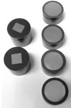
Figure 27. Material samples analyzed in SEM and EDS. To the right, samples from four main shafts. To the left, samples derived from excess material in an ingate system.
