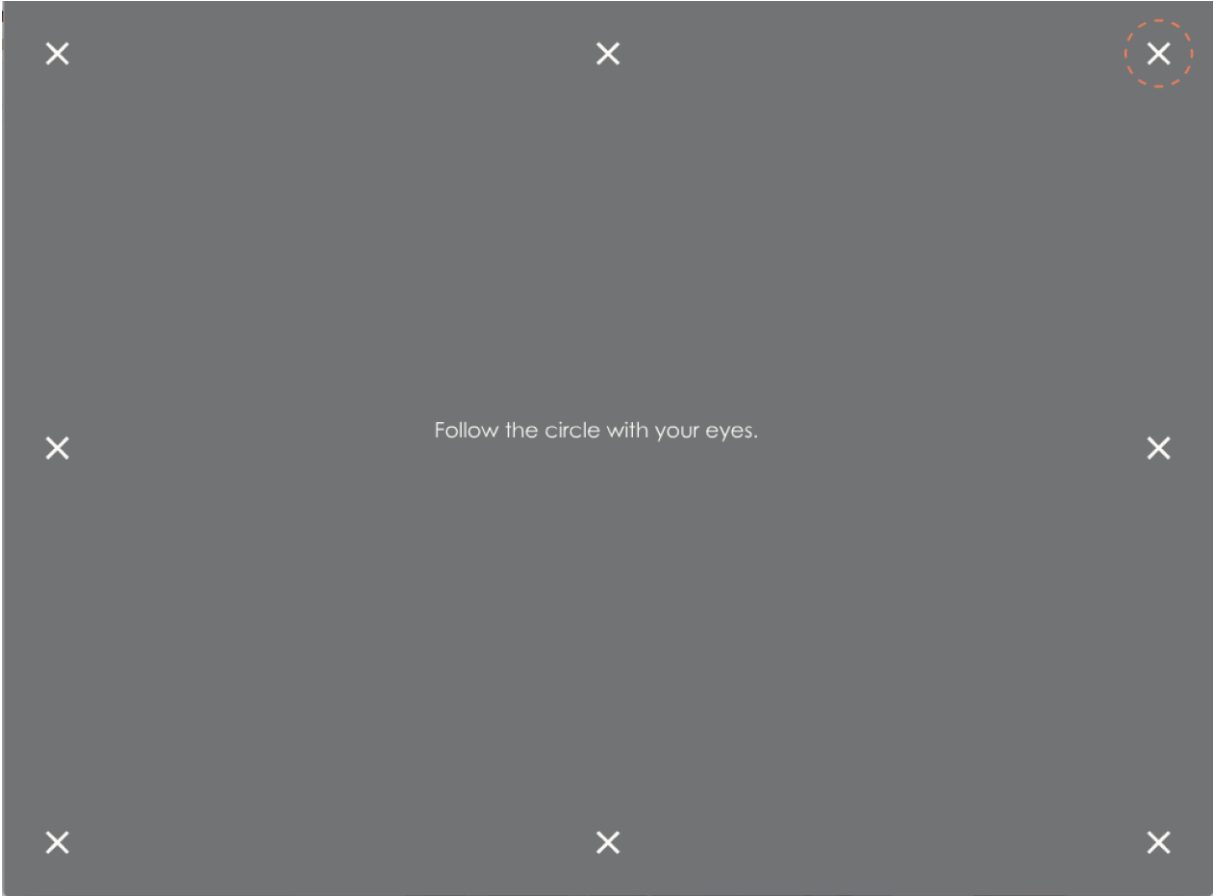
Figure 47. Calibration of the eye tracker. The user will follow a dot with their eyes to nine points on the screen.
