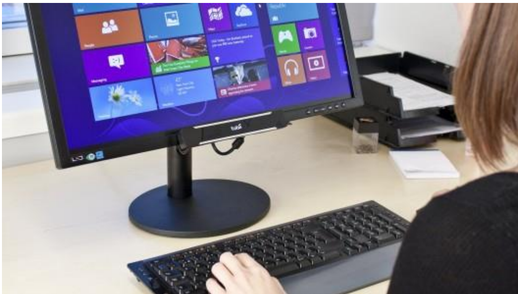
Figure 1. A remote eye tracker connected to a computer screen.
