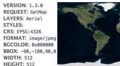
FIGURE 3.12: Example of WMS request parameters (left) and response (right). Image from the OnTerra WMS for Bing maps [16].
