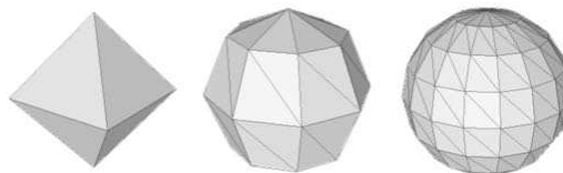
FIGURE 3.5: Tessellation from spherical coordinates. From the left; 4 width segments/2 height segments, 8 width segments/4 height segments, 16 width segments/8 height segments.
