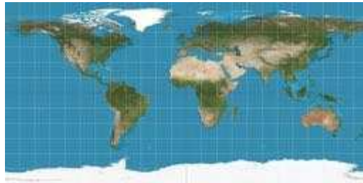
FIGURE 3.8: Example of an (equirectangular) cylindrical projection.
