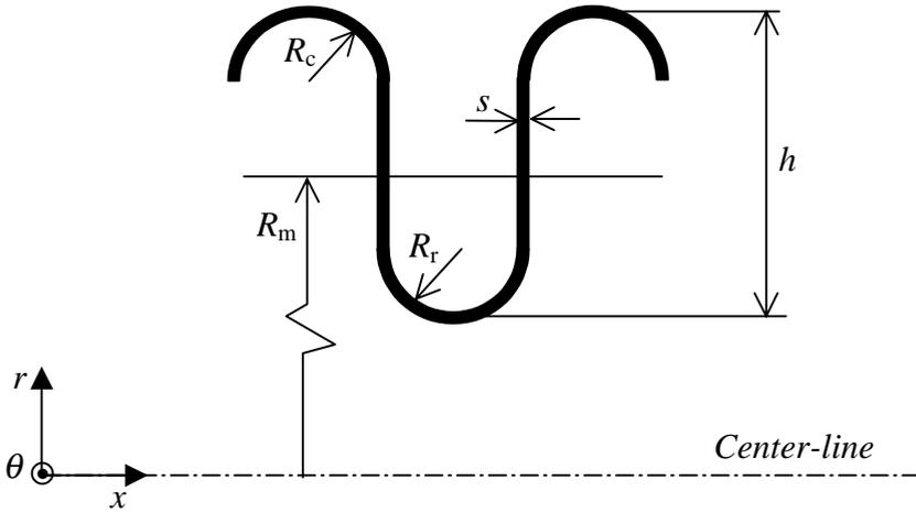
Figure 3.2. U-shaped convolution geometry.
