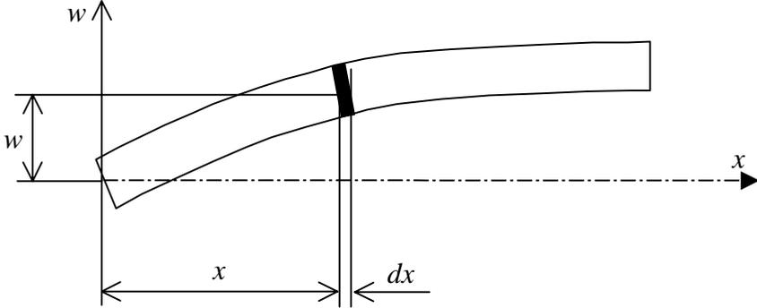
Figure 3.5. Displacements of bellows (pipe/beam) in bending vibration.
