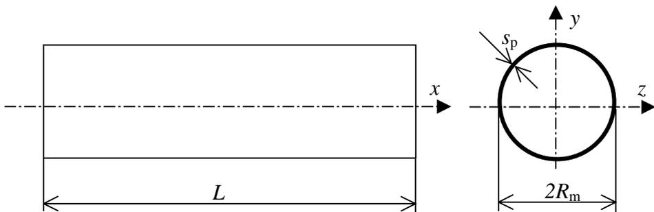
Figure 3.3. Thin-walled pipe analogy of bellows.
