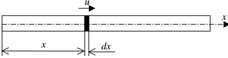
Figure 3.4. Displacements of bellows (pipe/rod) in axial vibration.
