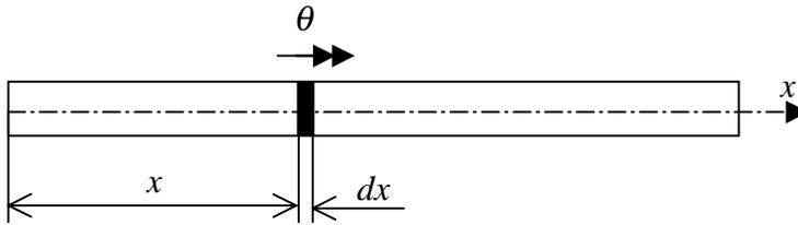
*Figure 3.6. Displacements of bellows (pipe/rod) in torsion vibration.*
