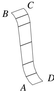
Figure 4.1. Shell element model of half convolution.
