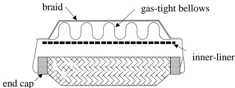
*Figure 3.1. Basic flexible connection design.*
