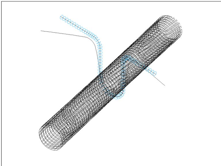
*Figure 4.6. First modes shape of original hanger on an exhaust pipe of length 500 mm.*
