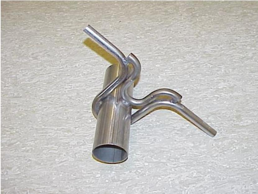
*Figure 4.10. Photo of prototype with pipe reinforcement.*
