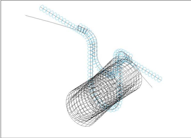
*Figure 4.7. First mode shape of the U-reinforced hanger on an exhaust pipe of length 144 mm.*
