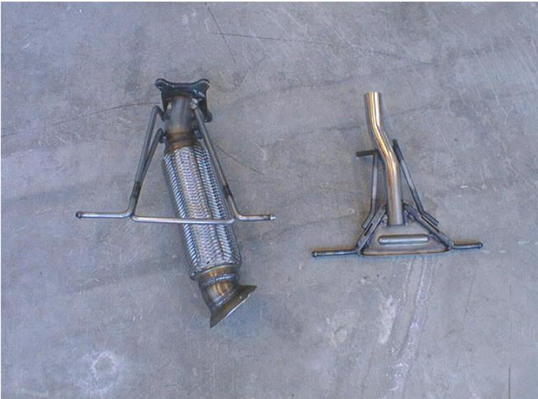
*Figure 3.2. Photo of Complicated hangers, case 2a mounted on a bellows and 2b without exhaust pipe.*
