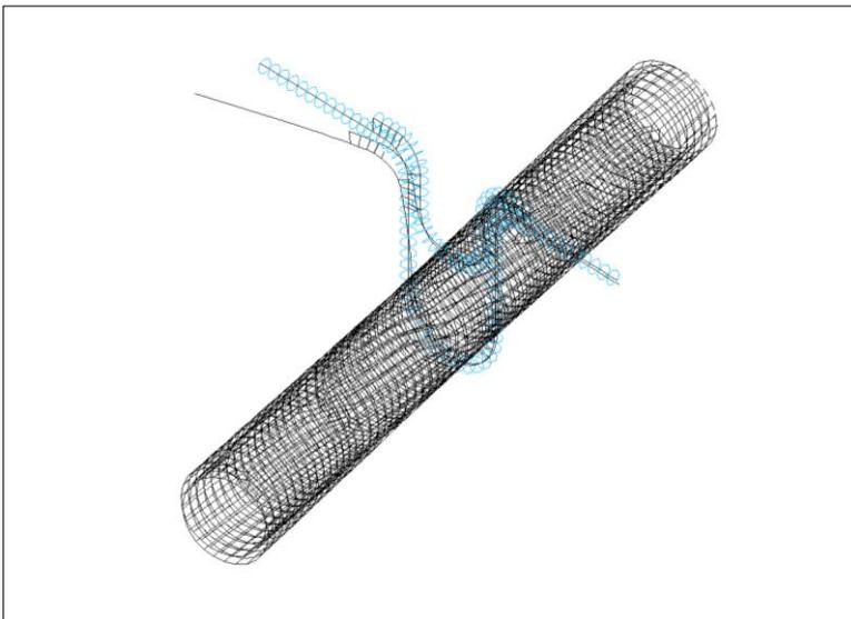
*Figure 4.8. First mode shape of the U-reinforced hanger on an exhaust pipe of length 500 mm.*
