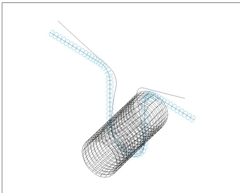
*Figure 4.3. First mode shape of the original hanger on an exhaust pipe of length 144 mm.*
