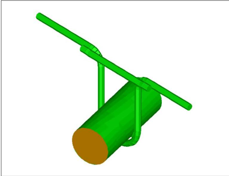
*Figure 4.4. T-reinforcement on the original hanger.*
