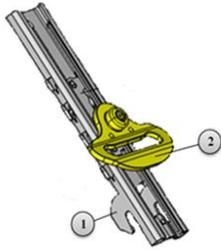
*Figure 2.1 Seat belt height adjuster.*
