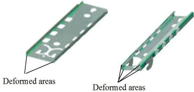
*Figure 2.2 Bending process of height adjuster.*
