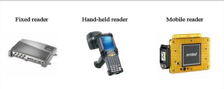
Figure 3.3: Types of RFID readers
