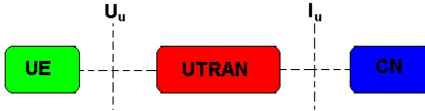
FIGURE 2.3 UMTS Main Reference Architecture
