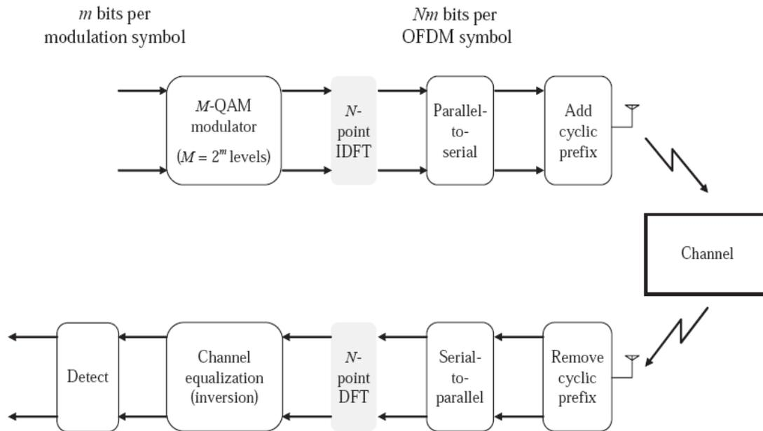
Figure 3-2 Basic OFDM transceiver [20].
