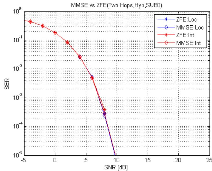
Figure 5-11 MMSE vs. ZFE equalization technique (Two Hops, Hybrid, SUB 0).
