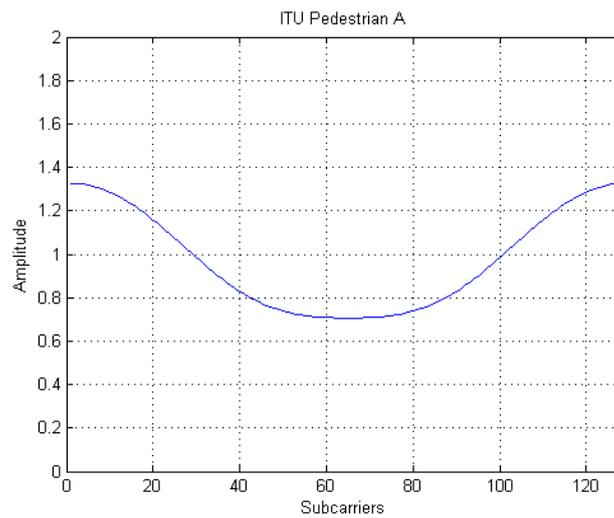
Figure 5-3 Frequency domain channel response of ITU Pedestrian A.
