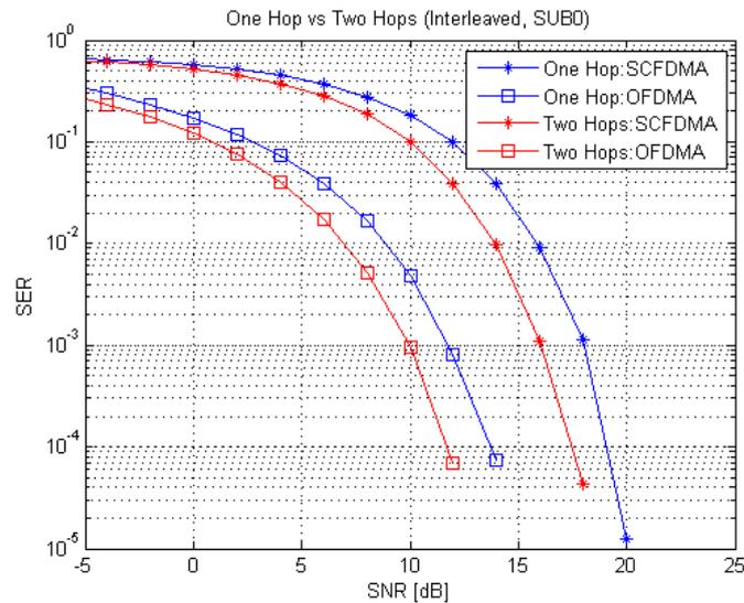
Figure 5-22 One hop vs. two hops (Interleaved, SUB 0).
