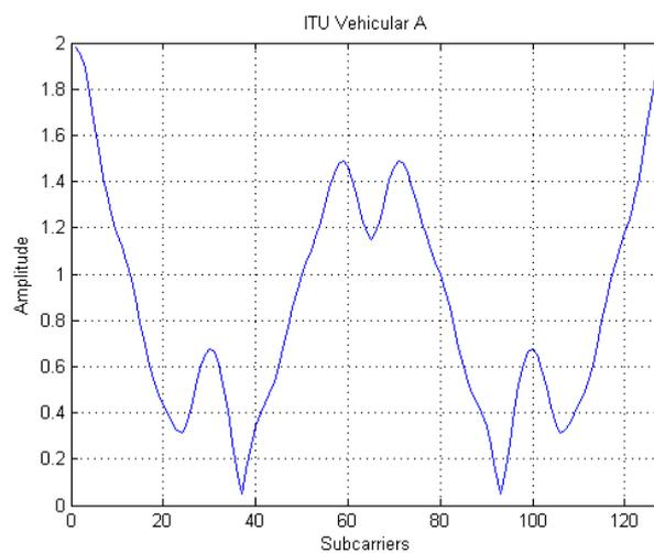
Figure 5-4 Frequency domain channel response of ITU Vehicular A.
