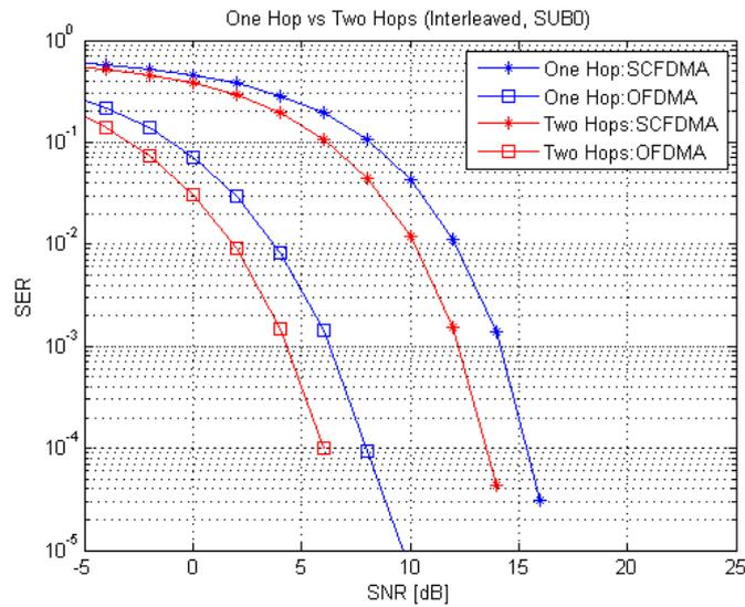
Figure 5-14 One hop vs. two hops (Interleaved, SUB0).
