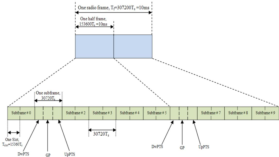
Figure 4-5 LTE frame structure Type 2 [28].
