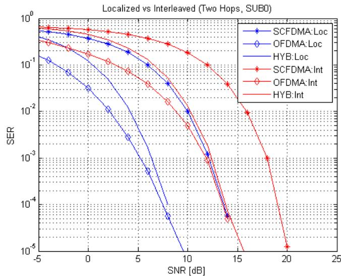
Figure 5-25 Localized vs. Interleaved subcarriers mapping (Two Hops, SUB 0).
