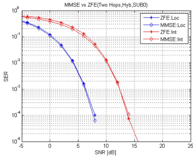
Figure 5-27 MMSE vs. ZFE equalization technique (Two Hops, Hybrid, SUB 0).
