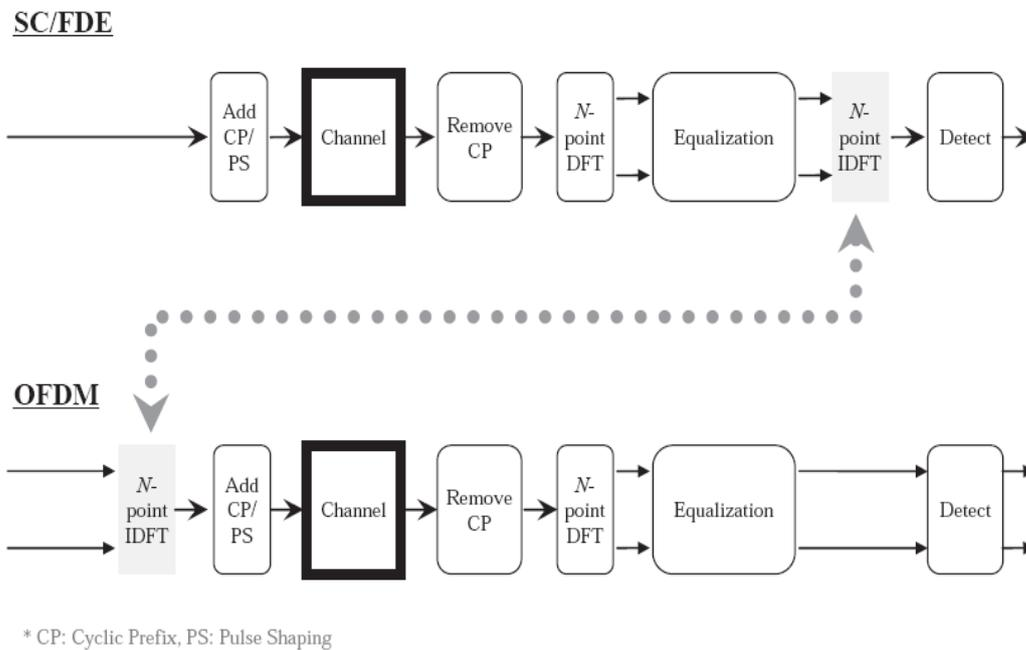
Figure 3-4 OFDM and SC-FDE transceiver comparison [20].
