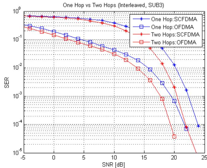
Figure 5-24 One hop vs. two hops (Interleaved, SUB 3).
