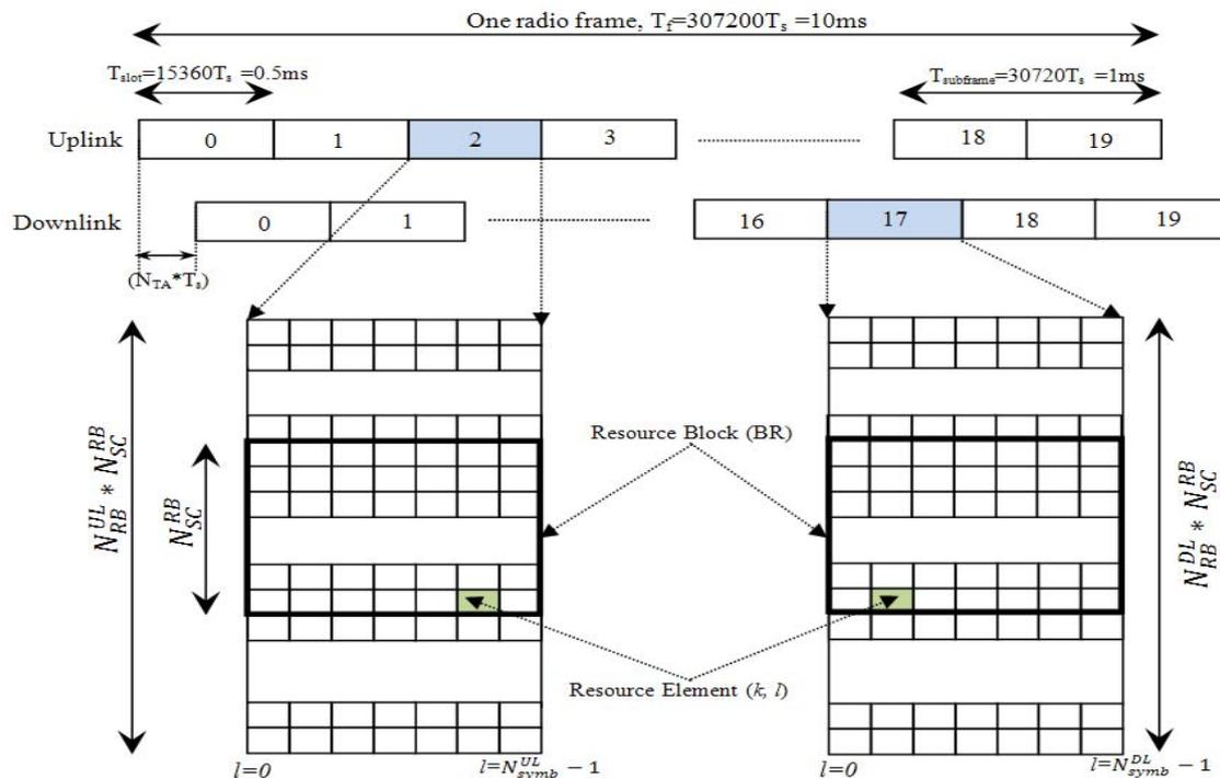
Figure 4-6 Frame structure and physical resource block in LTE uplink & downlink [7].
