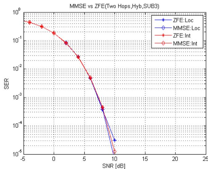
Figure 5-12 MMSE vs. ZFE equalization technique (Two Hops, Hybrid, SUB 3).
