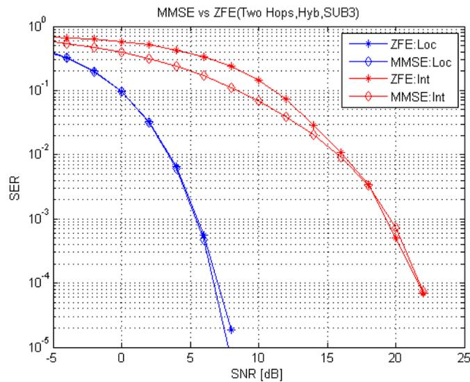
Figure 5-28 MMSE vs. ZFE equalization technique (Two Hops, Hybrid, SUB 3).
