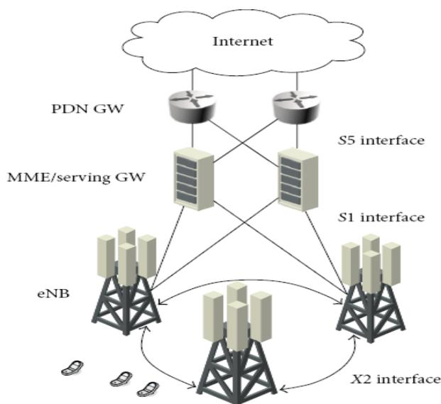
Figure 2-2 LTE Release 8 Network Architecture [1].
