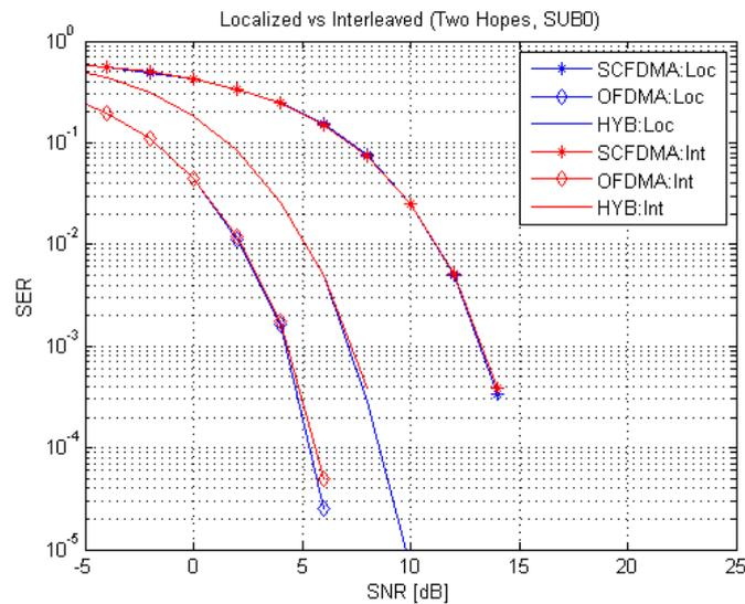
Figure 5-9 Localized vs. Interleaved subcarriers mapping (Two Hops, SUB 0).
