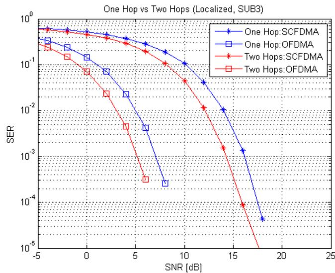
Figure 5-15 One hop vs. two hops (Localized, SUB 3).
