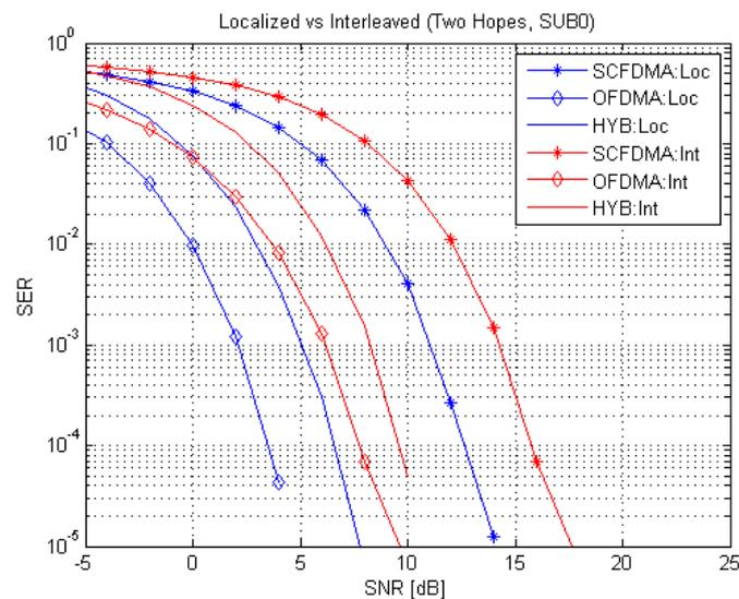
Figure 5-18 Localized vs. Interleaved subcarriers mapping (Two Hops, SUB 0).
