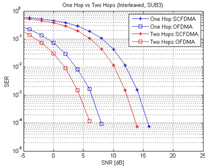
Figure 5-16 One hop vs. two hops (Interleaved, SUB 3).
