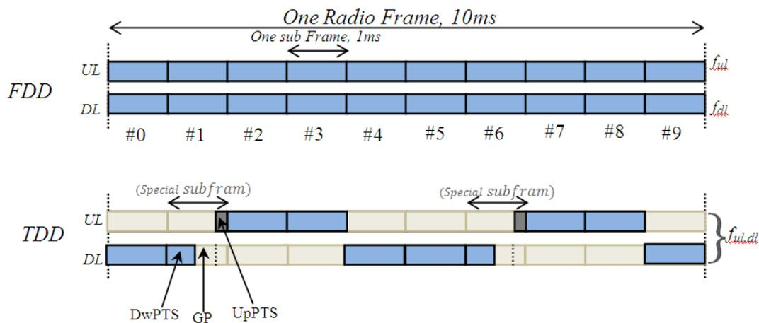
Figure 4-3 LTE frame structure in FDD and TDD modes [15].
