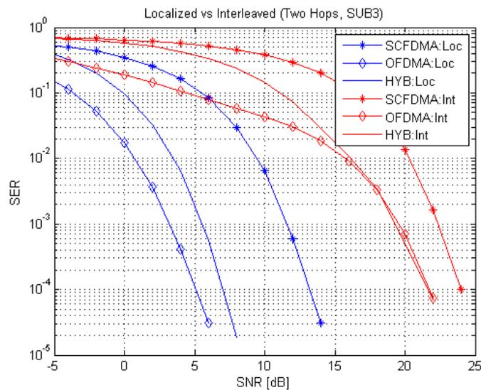
Figure 5-26 Localized vs. Interleaved subcarriers mapping (Two Hops, SUB 3).
