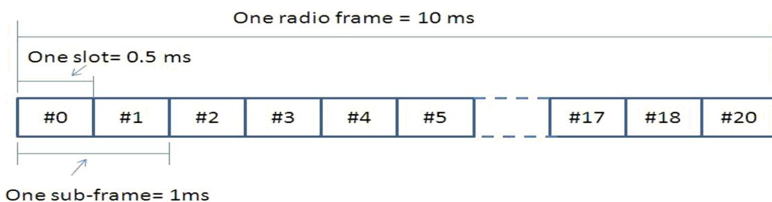
Figure 4-4 LTE frame structure Type1 [28].
