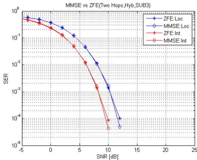
Figure 5-20 MMSE vs. ZFE equalization technique (Two Hops, Hybrid, SUB 3).
