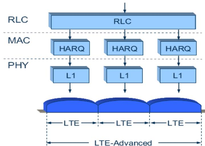
Figure 2-3 Carrier aggregation concept in LTE-Advanced [15].
