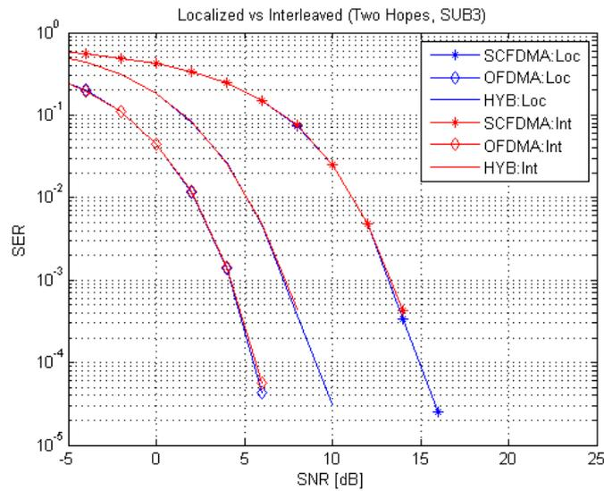
Figure 5-10 Localized vs. Interleaved subcarriers mapping (Two Hops, SUB0).
