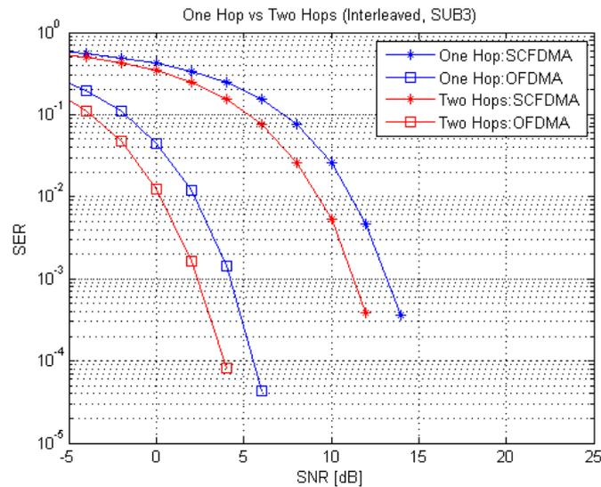
Figure 5-8 One hop vs. two hops (Interleaved, SUB 3).
