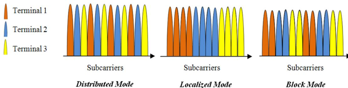
Figure 4-7 Basic subcarriers mapping schemes [25].
