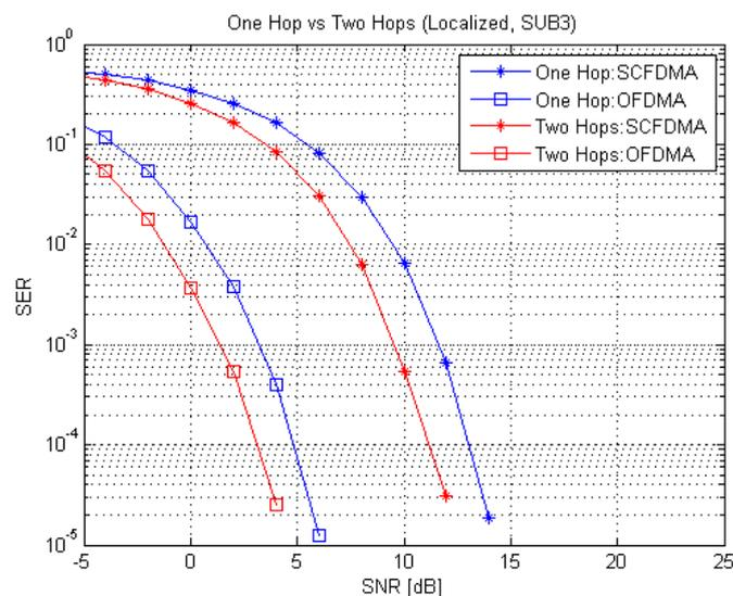
Figure 5-23 One hop vs. two hops (Localized, SUB 3).
