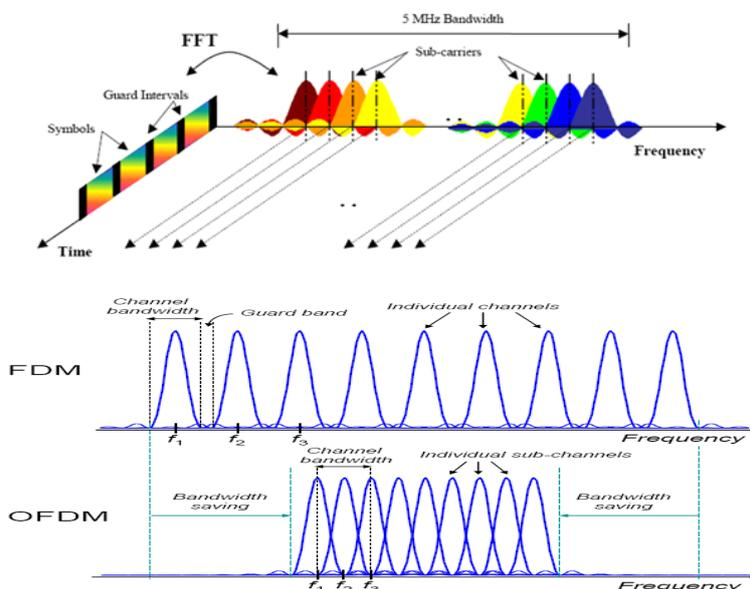
Figure 3-1 OFDM subcarriers overlapping [10].
