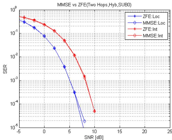
Figure 5-19 MMSE vs. ZFE equalization technique (Two Hops, Hybrid, SUB 0).
