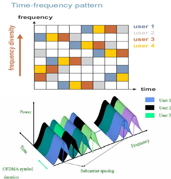
Figure 4-1 OFDMA basic operation [27].
