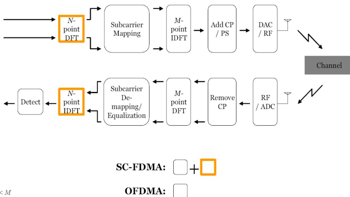
Figure 4-2 OFDMA and SC-FDMA transceiver comparison [25].
