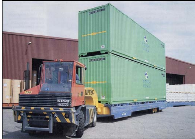
Figure 7-10: Truck with Cassette with Two Containers of 40' One upon the Other Source: http://www.tts-marine.no , “TTS Group”.
