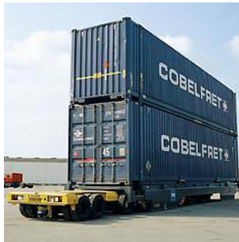
Figure 7-11: IPSI AGV with Cassette with Two Containers of 40' One upon the Other Source: http://www.tts-marine.no , “TTS Group”.
