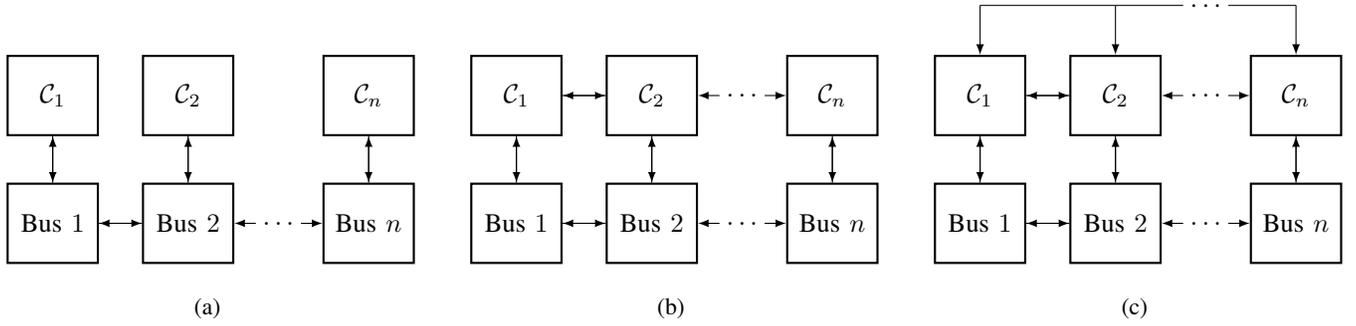
Figure 1: (a) shows the decentralized architecture of the voltage droop controller (VDM). (b) shows the distributed architecture of Controllers (I) and (III). (c) shows the architecture of Controller (II), with all-to-all communication.
