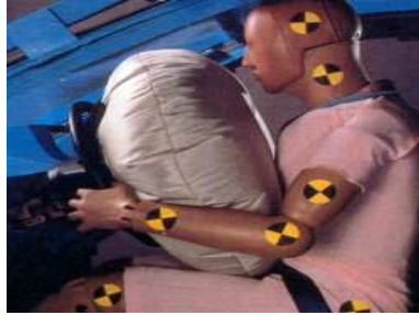
Figure 1.3: Inflated membrane as airbags ( http://www.carsp.ca )
