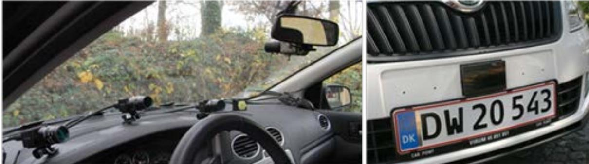
*Figure 1: The 3-camera system for tracking eye movements together with the scene camera behind the rear view mirror (photo left). The scanner is installed in front of the car (photo right).*
