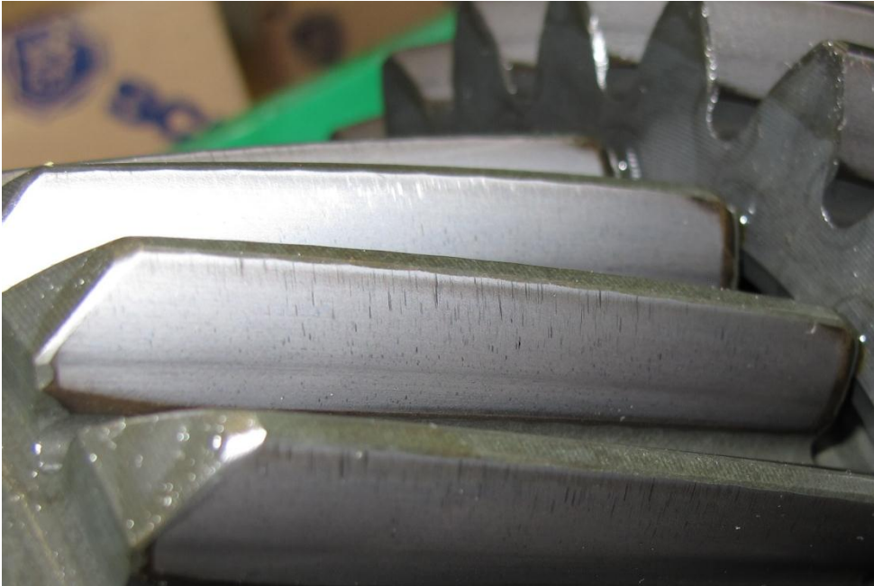
Figure 45, Scuffing marks seen on surface of middle tooth close to the tip (Courtesy Scania)
