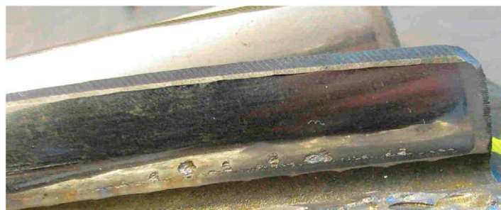
Figure 43, Photograph showing “pitting” line in tip relief area on same helical gear (Courtesy Scania)
