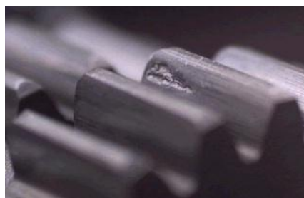
Figure 10, Pitting on a gear surface (Courtesy Scania)
