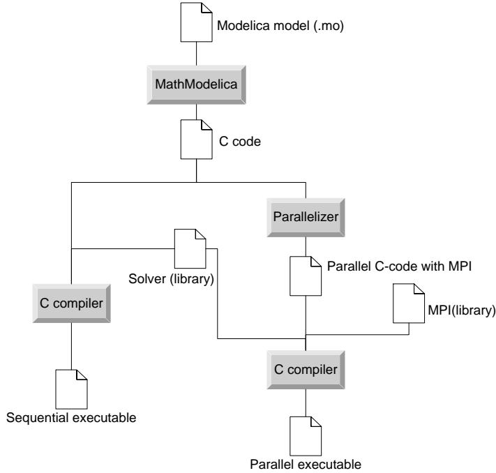
**Fig. 4.** The architecture of a Modelica simulation environment
