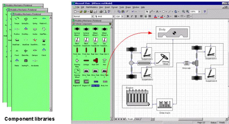
**Fig. 2.** Visual component based modeling in MathModelica.
