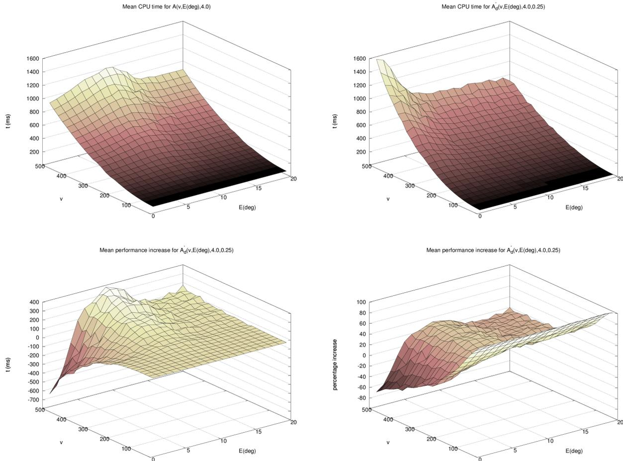
**Figure 3.** Comparison of performance when separating static and dynamic variables. The ratio of dynamic variables is fixed at  $r = 0.25$ . The top two graphs show the mean absolute CPU times and the bottom two graphs show the mean absolute and relative performance increase.
