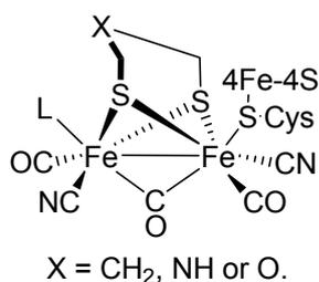
**Figure 4.3** The consensus structure of the active site of Fe-Fe Hydrogenase.
