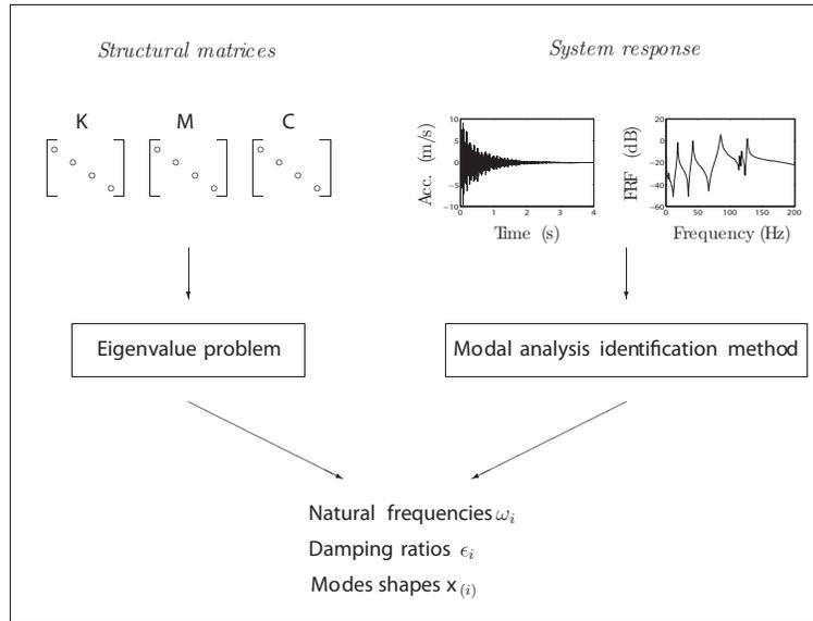
Figure 2.1: Theoretical and experimental modal analysis reproduced from [www.ltas-vis.ulg.ac.be](http://www.ltas-vis.ulg.ac.be)
