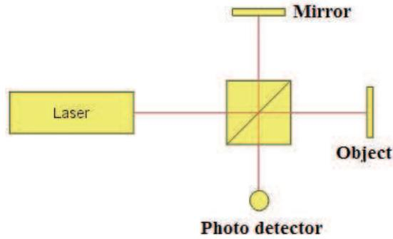
Figure 5.3: Laser Vibrometer Setup reproduced from [www.aplv.blogspot.se](http://www.aplv.blogspot.se)
