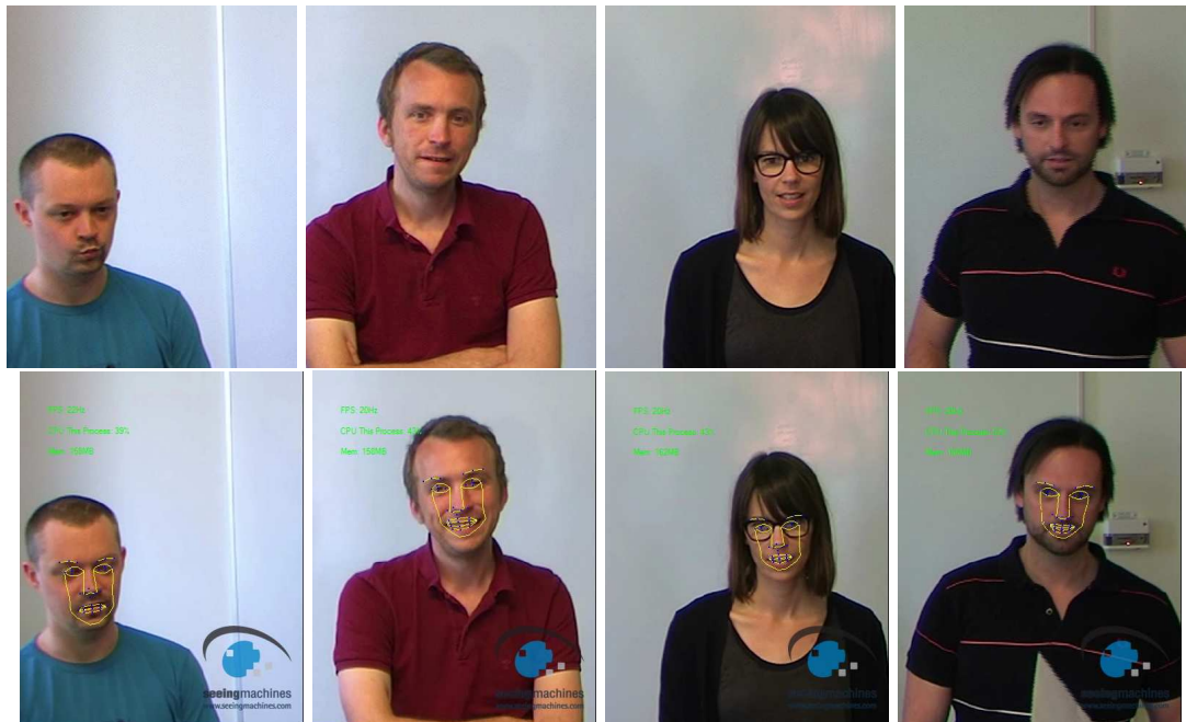
Figure 3.4: Tracking of FaceAPI on the cropped images. In upper figure, a frame of the dialogue video showing the different speakers separated manually into different parallel video files and in lower figure, a frame of the dialogue video showing the faceAPI tracking on the different speakers.
