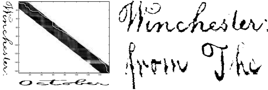
Fig. 3. Right: Illustration of the Sakoe-Chiba constraint on the weight matrix in dynamic time warping. Only the diagonal part of the weight matrix is considered valid for warping (diagonal \pm 15 elements). The lowest cost path (white line) through the diagonal band represent the warping. Left: Three segmented, binarized and normalized words from the Washington database, used in our evaluation. Note the unnatural slant on the “f” in “from.” This is because letters are normalized according to the dominant slant.
