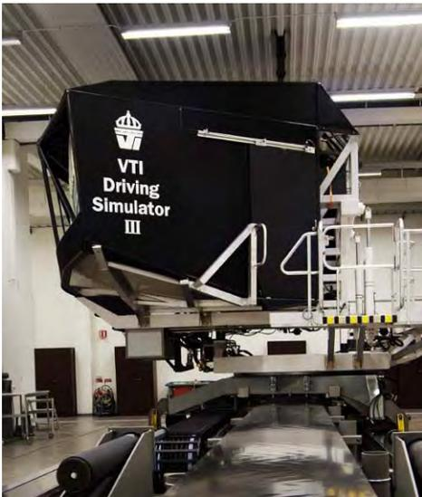
Figure 1 Moving base driving simulator at VTI.
