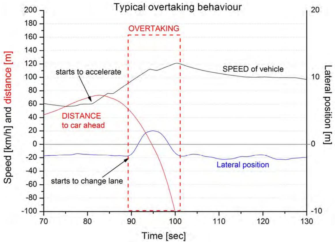
Figure 35 Typical overtaking plotted. Lateral position of own car, distance to car ahead and speed of own car are shown.
