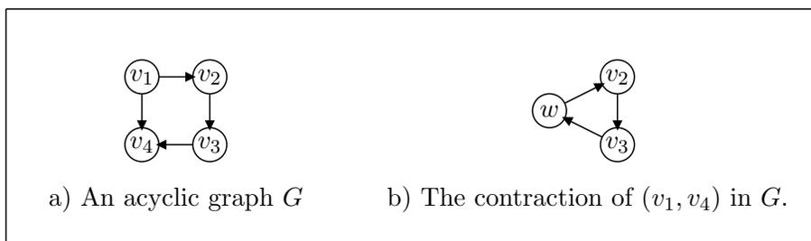
Figure 7: Contracting an edge in an acyclic graph can result in a cycle.
