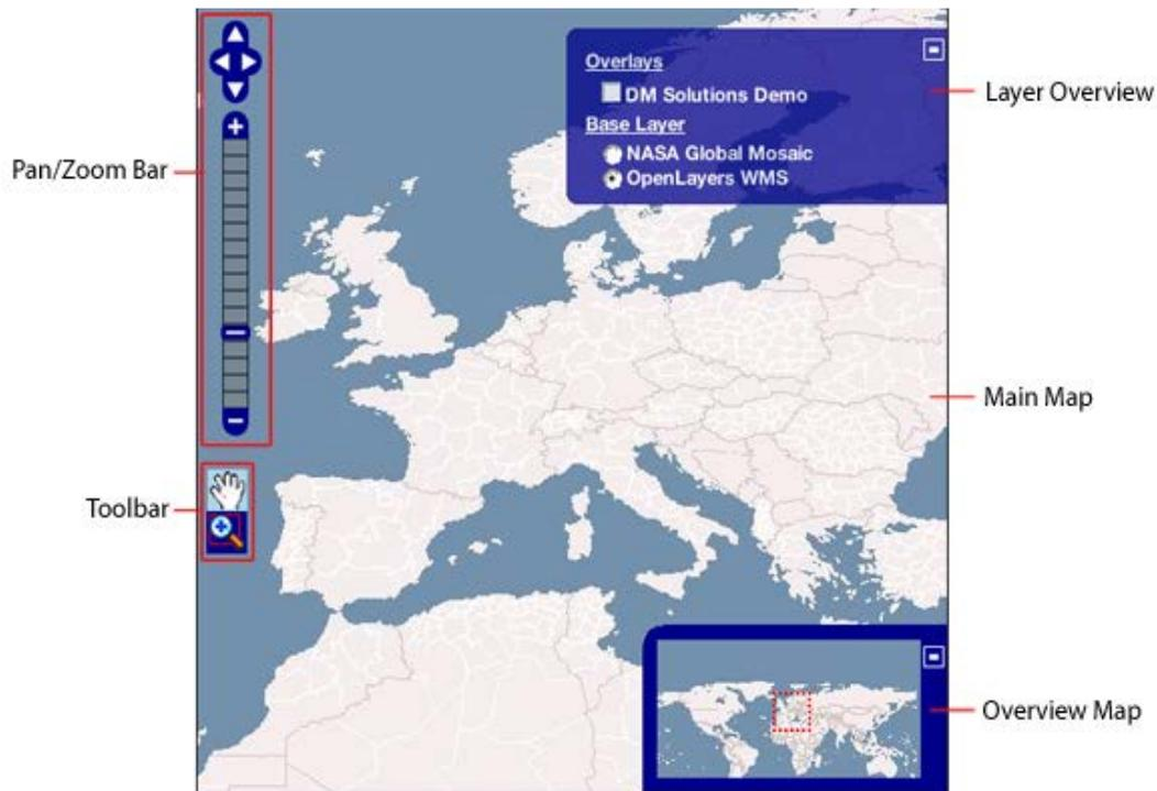
Figure 5. Components of Web Mapping Application OpenLayers (Schütze, Web Mapping, 2007)
