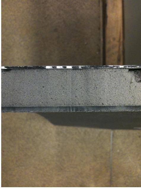
Figure 3.2: From top to bottom, the aluminium plate, the porous layer and the rubber plate.
