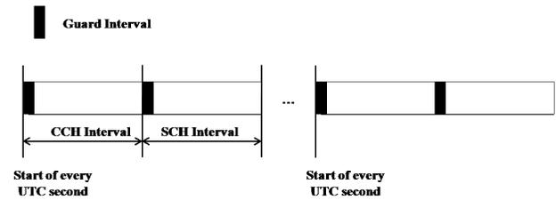
Fig. 1. The WAVE channel switching
