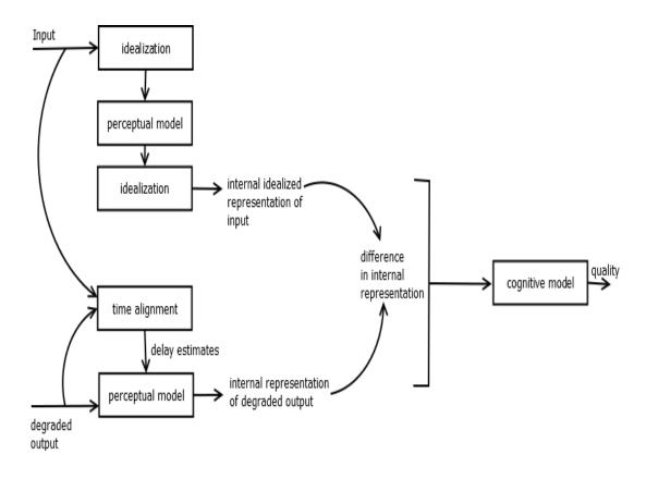
Figure 2. Basic overview of ITU-T P.863, POLQA. The computer model comprises a perceptual and a cognitive model (taken from [1]).
