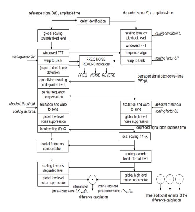
Figure 4. ITU-T P.863, POLQA - Perceptual model (Taken from [1]). Difference function is calculated in four different flavors.
