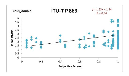
Figure 16. Correlation between subjective intelligibility scores and standard ITU-T P.863 output in super wideband mode for the 'Cous\_double' database. There were 196 degraded '/C/ous' words, the degradations used were: reduced playback level, bandwidth limitation, background noise, time-clipping and pulse distortion.
