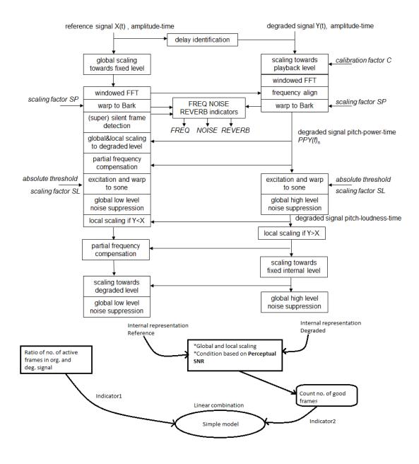
Figure 17. Integration of the simple model in ITU-T P.863 perceptual model. A linear combination of Indicator1 and Indicator2 is used as the model to predict individual CVC intelligibility scores. Cognitive model of ITU-T P.863 is totally discarded.
