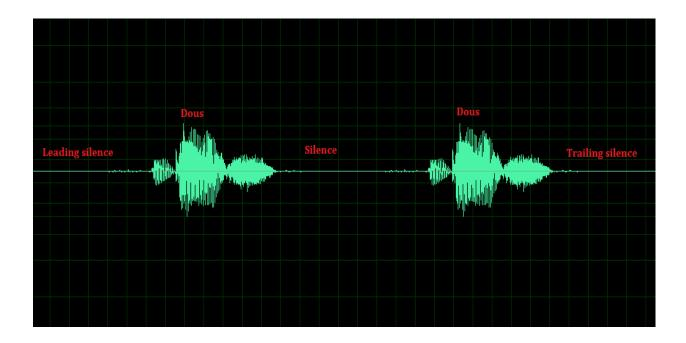
Figure 15. 'Dous\_ double' reference speech signal. Leading silence, trailing silence and the silent interval between two 'Dous' words are shown.
