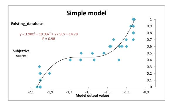
Figure 21. Correlation between the subjective scores and the model output values for an existing database at TNO. An excellent correlation of 0.98 is obtained. A total of 81 degraded speech signals suffering from severe time-clipping distortion were present in the database.
