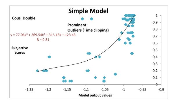
Figure 19. Correlation between the subjective scores and the model output values for 'Cous\_double' database. A reasonably good correlation of 0.81 is obtained. There were 196 degraded '/C/ous' words, the degradations used were: reduced playback level, bandwidth limitation, background noise, time-clipping and pulse distortion.
