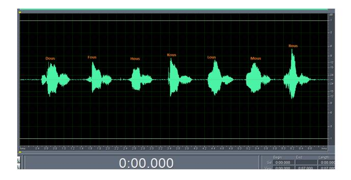
Figure 8. A recorded 'C/ous/' file from a source. It contains seven different CVC words. This file is pre-filtered and leveled before extracting individual CVC words.
