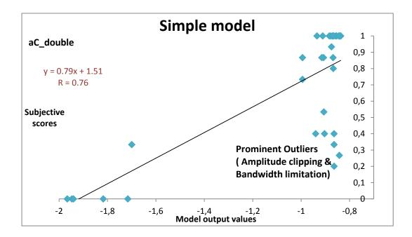
Figure 20. Correlation between the subjective scores and the model output values for  $'aC_{-}$ double' database. This database does not contain 'aH' words. A total of 36 degraded 'a/C/' words were present in the database. The degradations used were: background noise, bandwidth limitation, time-clipping, amplitude-clipping and codec distortions. A reasonably good correlation of 0.76 is obtained.
