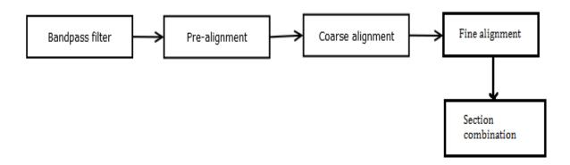
Figure 3. Five major blocks of the Temporal Alignment algorithm used in ITU-T P.863, POLQA (Redrawn from [8]).
