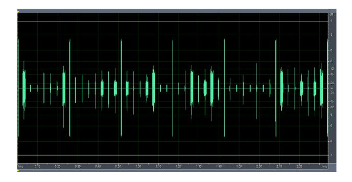
Figure 10. Concatenated audio file used for a listening test. A silence of 2 seconds is added after every degraded '/C/ous' word.
