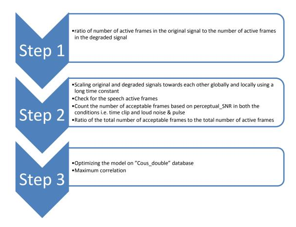
Figure 18. A flowchart illustrating the simple model.
