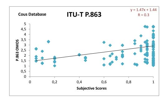
Figure 14. Correlation between subjective intelligibility scores and standard ITU-T P.863 output in super wideband mode for the '/C/ous' database. There were 196 degraded '/C/ous' words, the degradations used were: reduced playback level, bandwidth limitation, background noise, time-clipping and pulse distortion.
