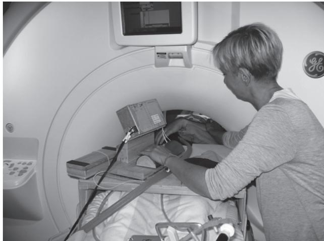
**Figure 1.** The touch device in the scanner room indicated the different touch conditions, the correct force (2.5 N) and the correct velocity (1–5 cm/s). The force of the mirror movement applied on the dummy arm was measured by force transducers and sampled in a computer.
