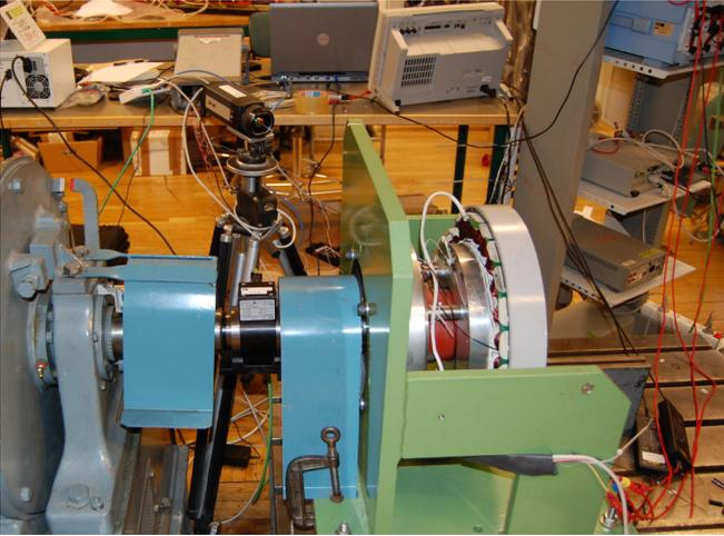
Fig. 4. Thermal measurement setup of the investigated outer-rotor PMSM.
