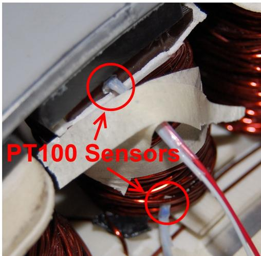
Fig. 5. PT100 temperature sensors mounted on the front side of the stator tooth tip and on the winding coil.
