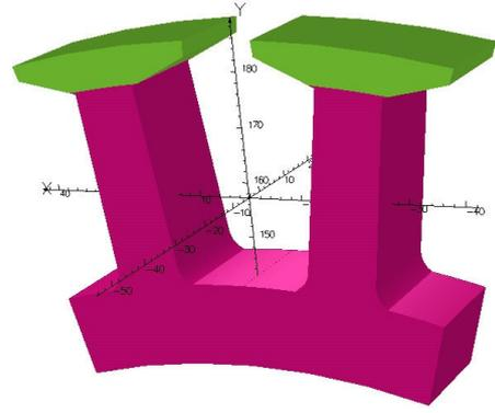
Fig. 2. Stator tooth tips (green) and stator tooth yoke (violet).
