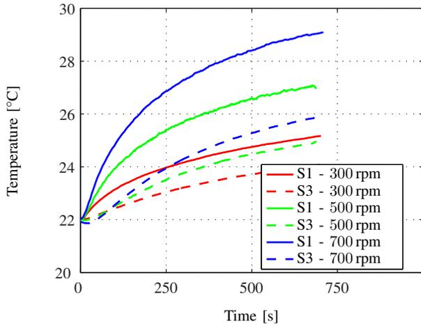
Fig. 7. Temperature rises of Sensor 1 (S1) and Sensor 3 (S3) at no-load condition for 300 rpm, 500 rpm and 700 rpm.
