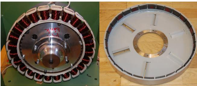
Fig. 1. Stator and rotor of the investigated outer-rotor PMSM.
