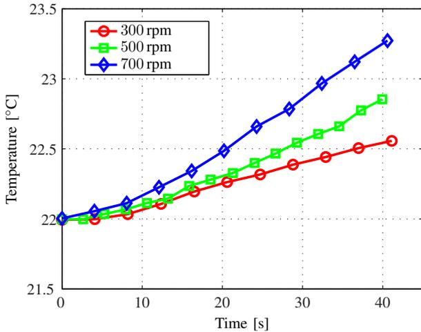
Fig. 8. Initial temperature rise of sensor 1 for 300 rpm, 500 rpm and 700 rpm.
