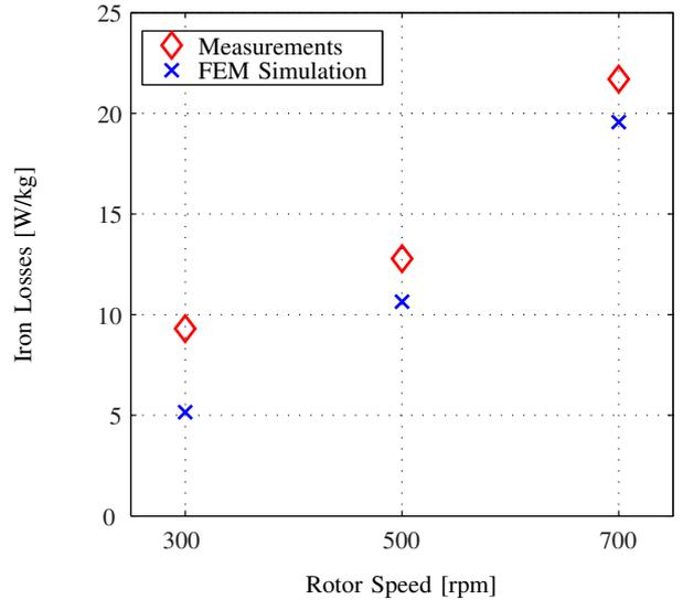
Fig. 9. Iron loss density in the stator tooth tips determined by FEM calculations and thermal measurements for 300 rpm, 500 rpm and 700 rpm.
