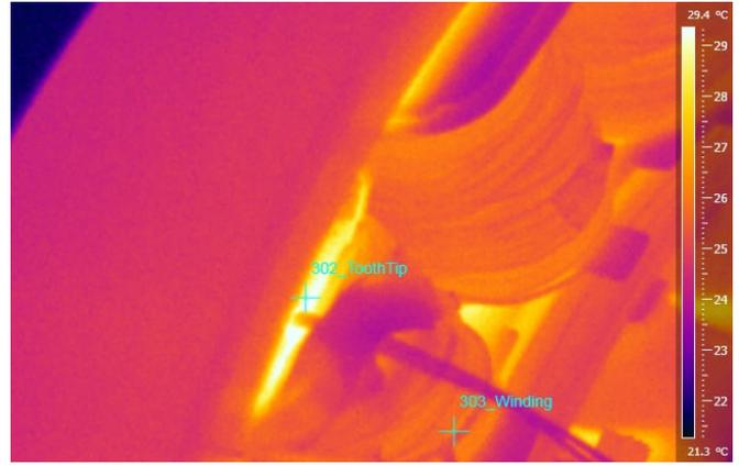
Fig. 6. Thermal image of the stator coils and mounted PT100 sensors at a no-load test with 700 rpm.
