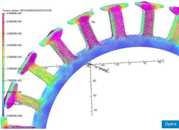
Fig. 3. Iron loss density (surface contour in W/kg) and current density vectors at no-load, 700 rpm.
